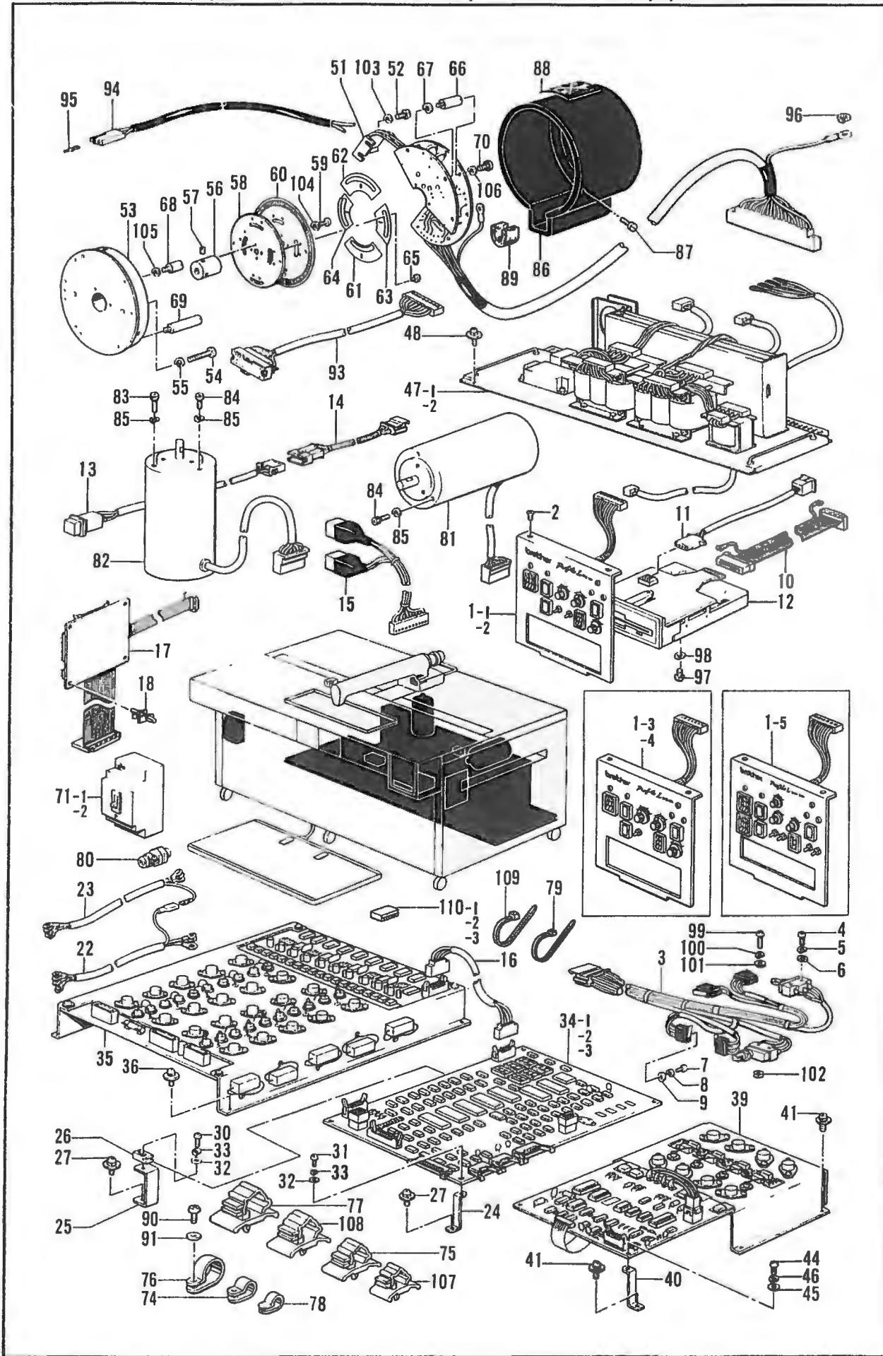
P. 電気品関係 / Power supply equipment mechanism / Stromversorgung /
