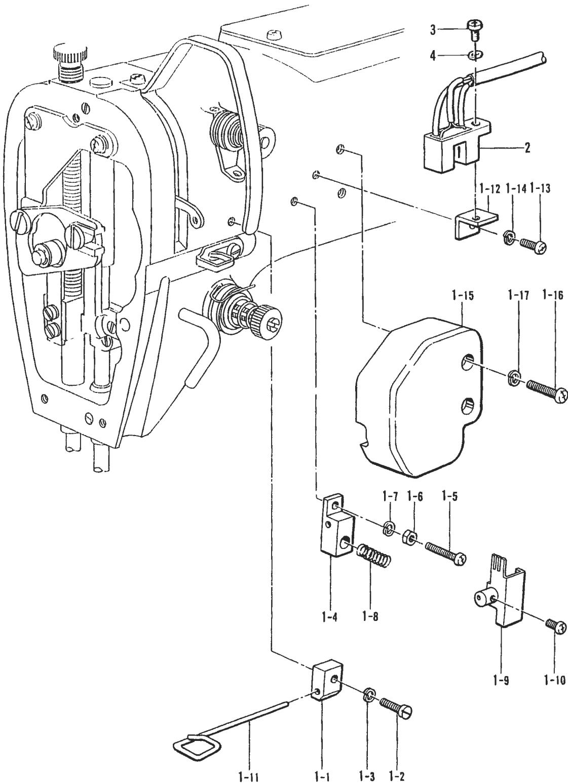
1. 糸切れ感知関係 (オプション) / Thread breakage detector mechanism (option)/
