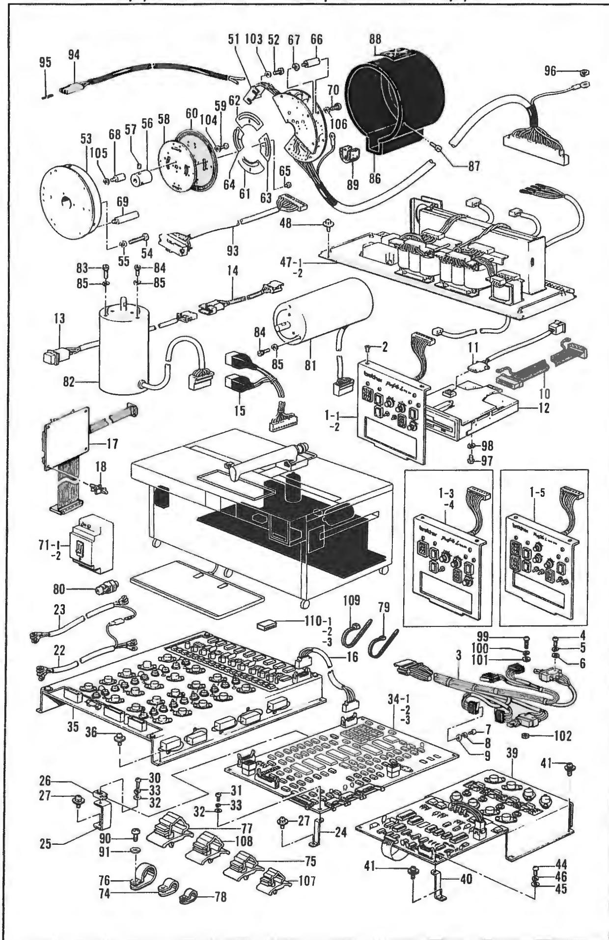
P. 電設品関係/Power supply equipment mechanism/Stromversorgung/
