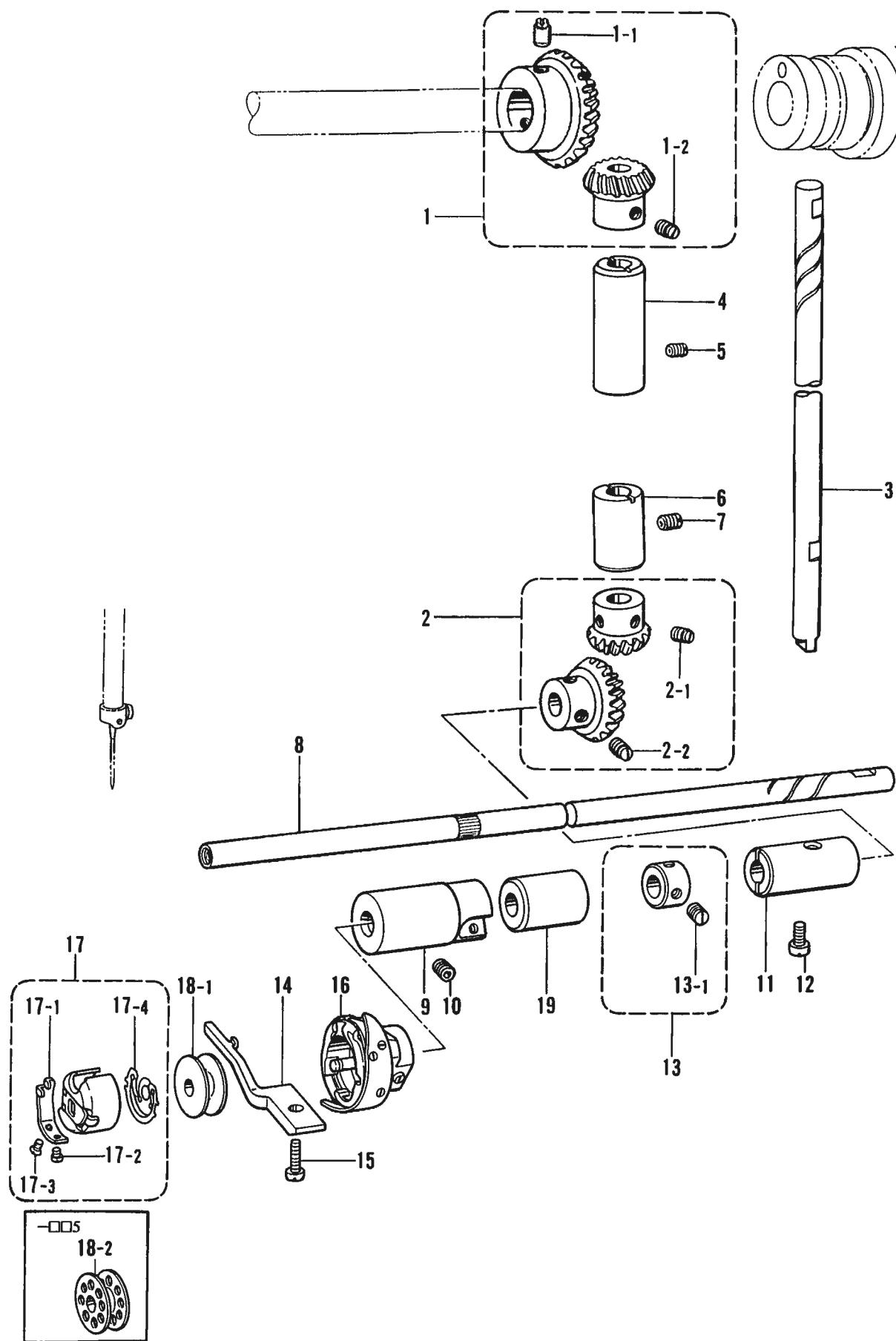
G. カマ関係/Rotary hook mechanism/Greifervorrichtung/
