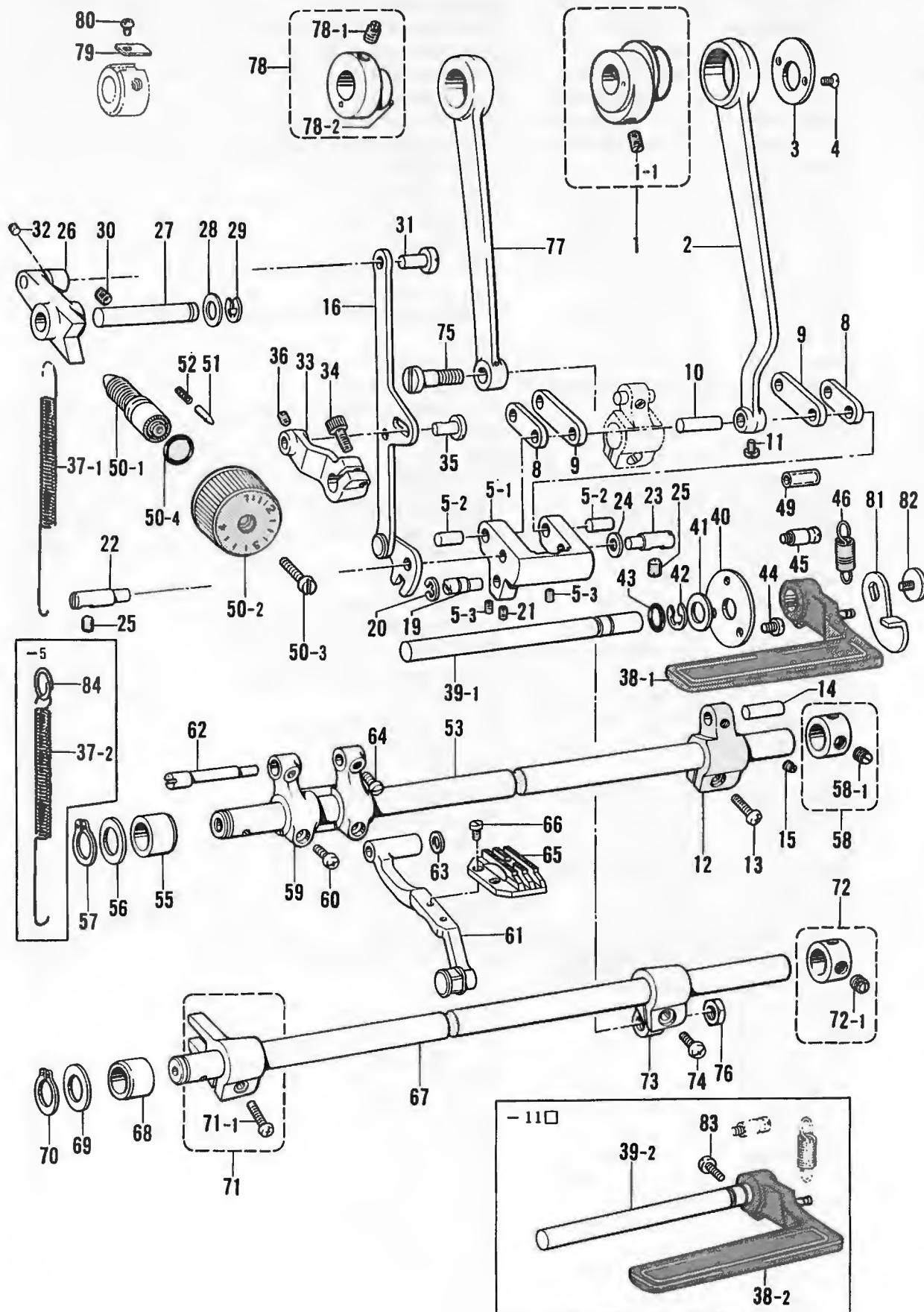
E. 送り関係 / Feed mechanism / Transportvorrichtung /
