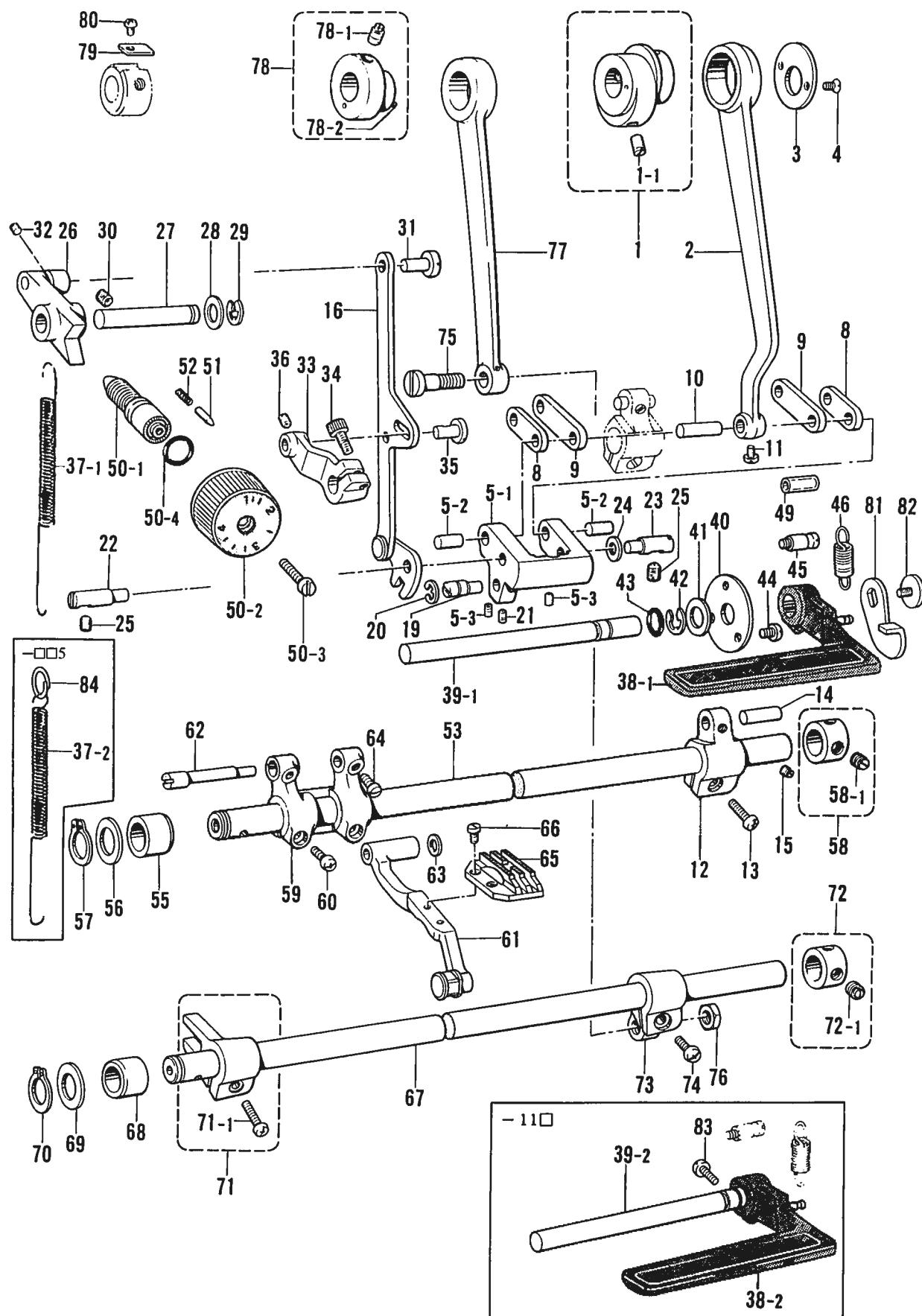
E. 送り関係/Feed mechanism/Transportvorrichtung/
