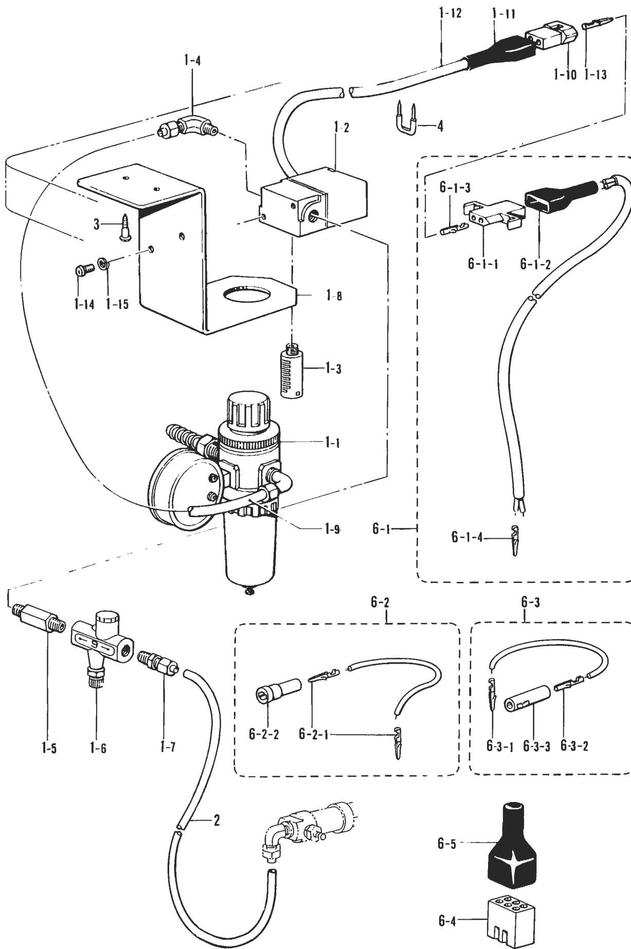
T. 空圧関係/Air pressure mechanism/Luftdruck/
