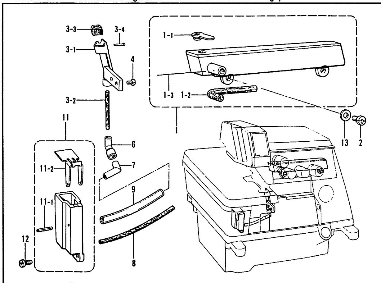
B. 駆動軸関係/Crank shaft mechanism/Kurbelwelle/
