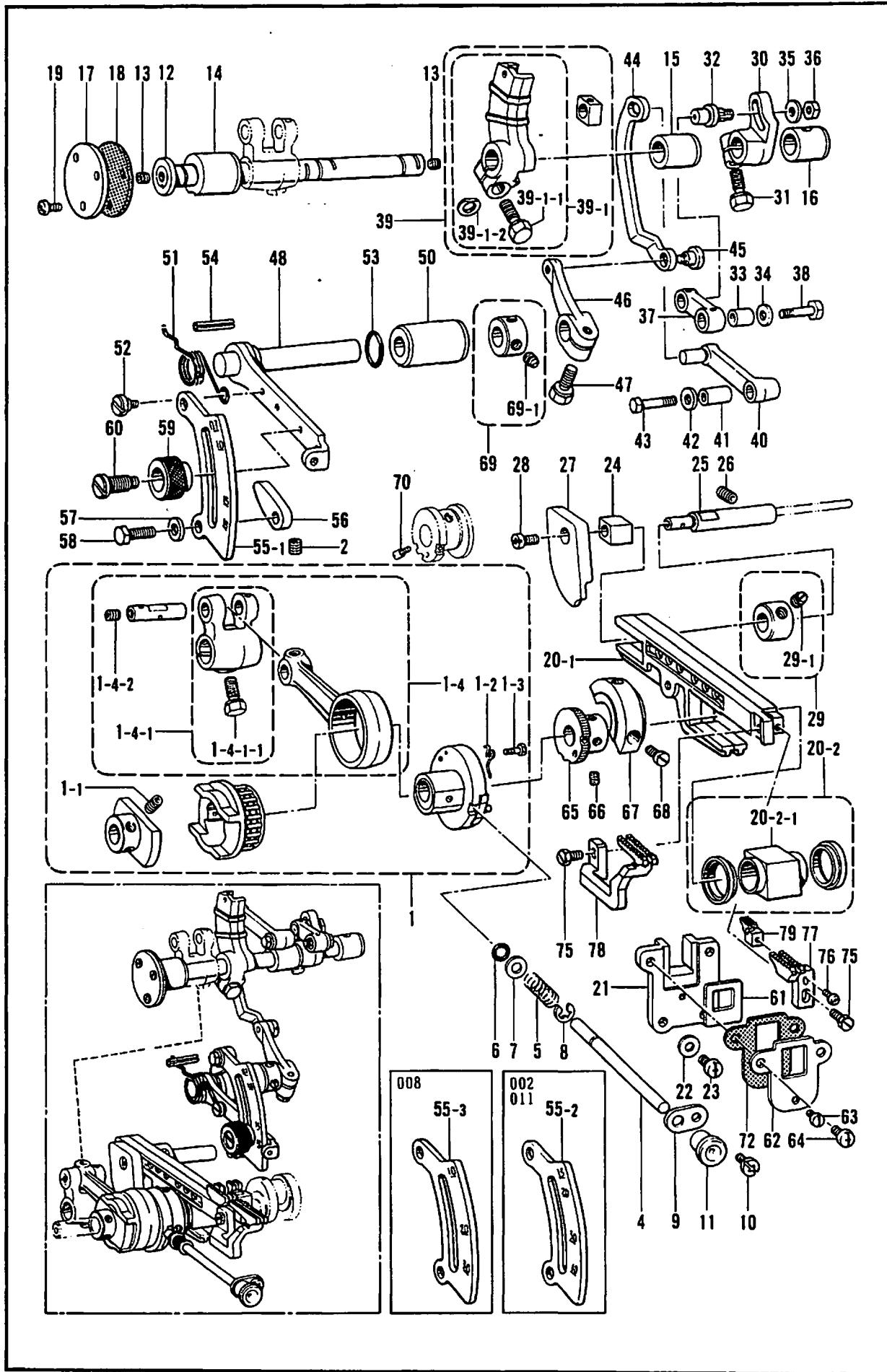
F. 送り関係/Feed mechanism/Transportvorrichtung/
