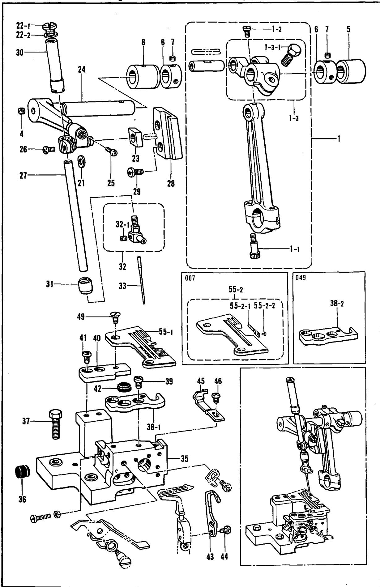
D. 針棒関係/Needle bar mechanism/Nadelstangenvorrichtung/
