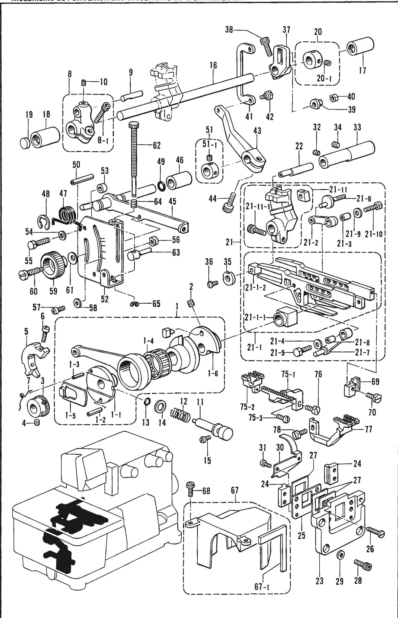
E. 送り関係/Feed mechanism/Transportvorrichtung/
