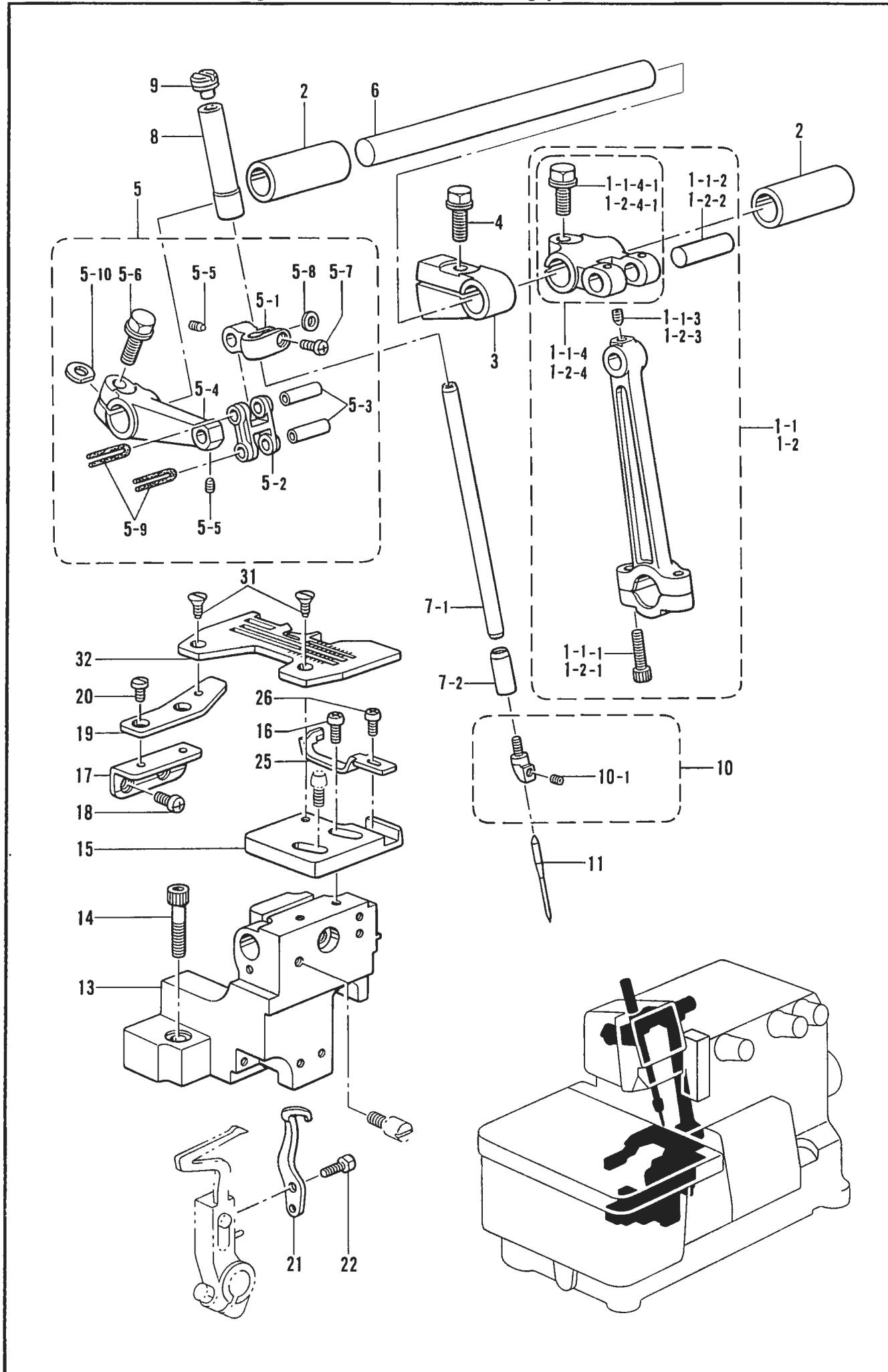
C. 針棒関係 /Needle bar mechanism/Nadelstangenvorrichtung/
