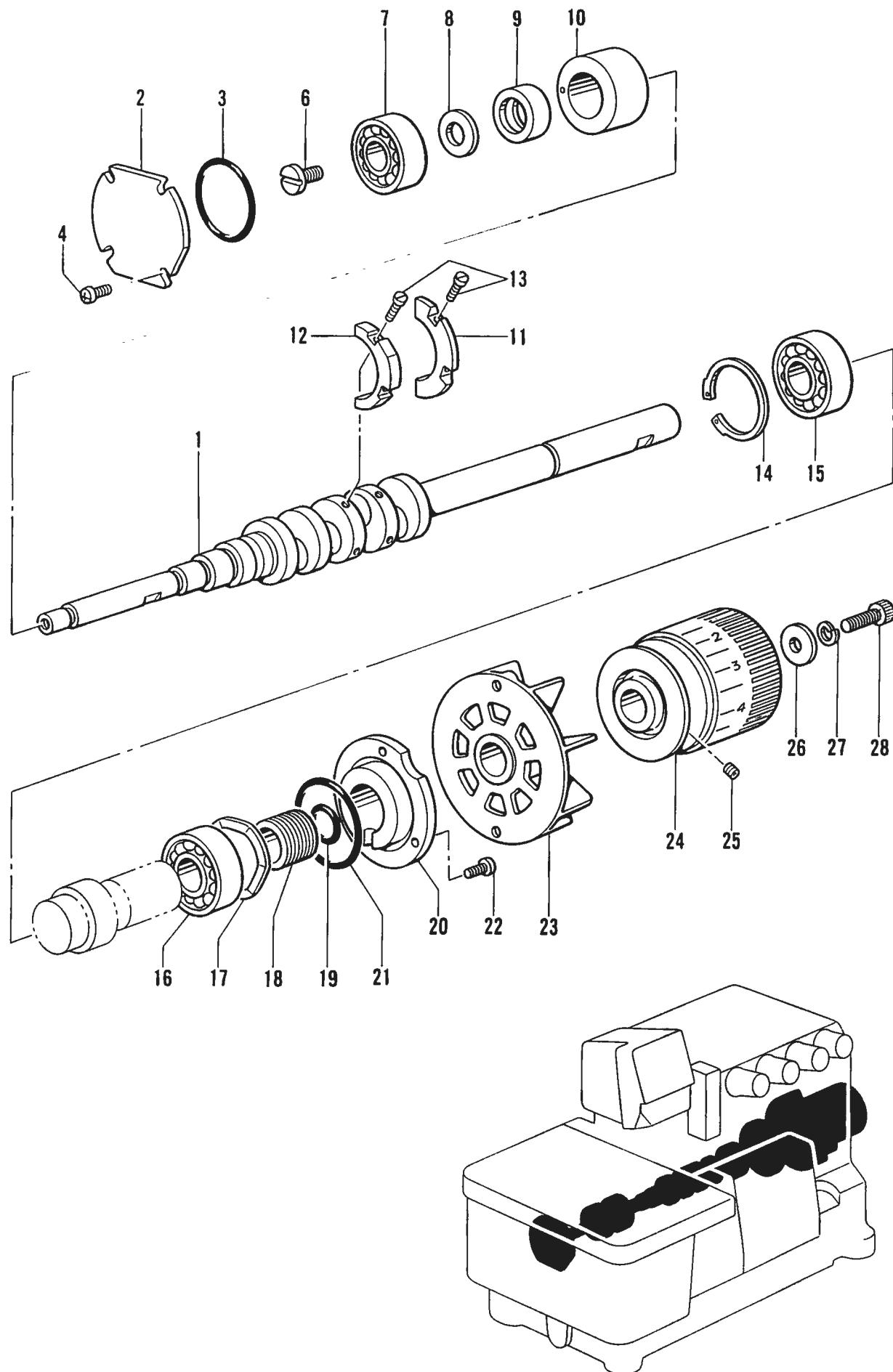
B. 駆動軸関係/Crank shaft mechanism/Kurbelwelle/
