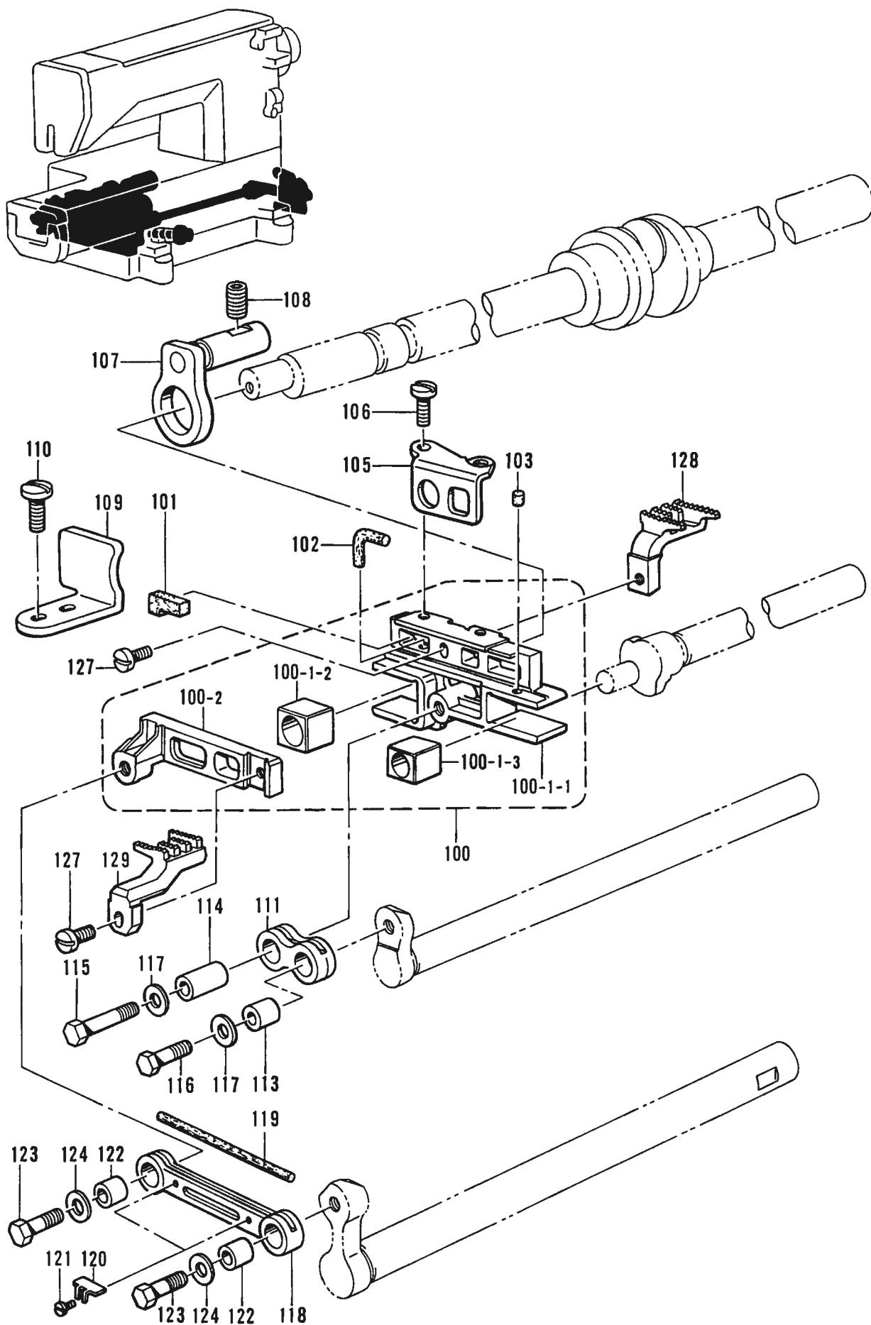
**E2. 送り関係/Feed mechanism/Transportvorrichtung/
