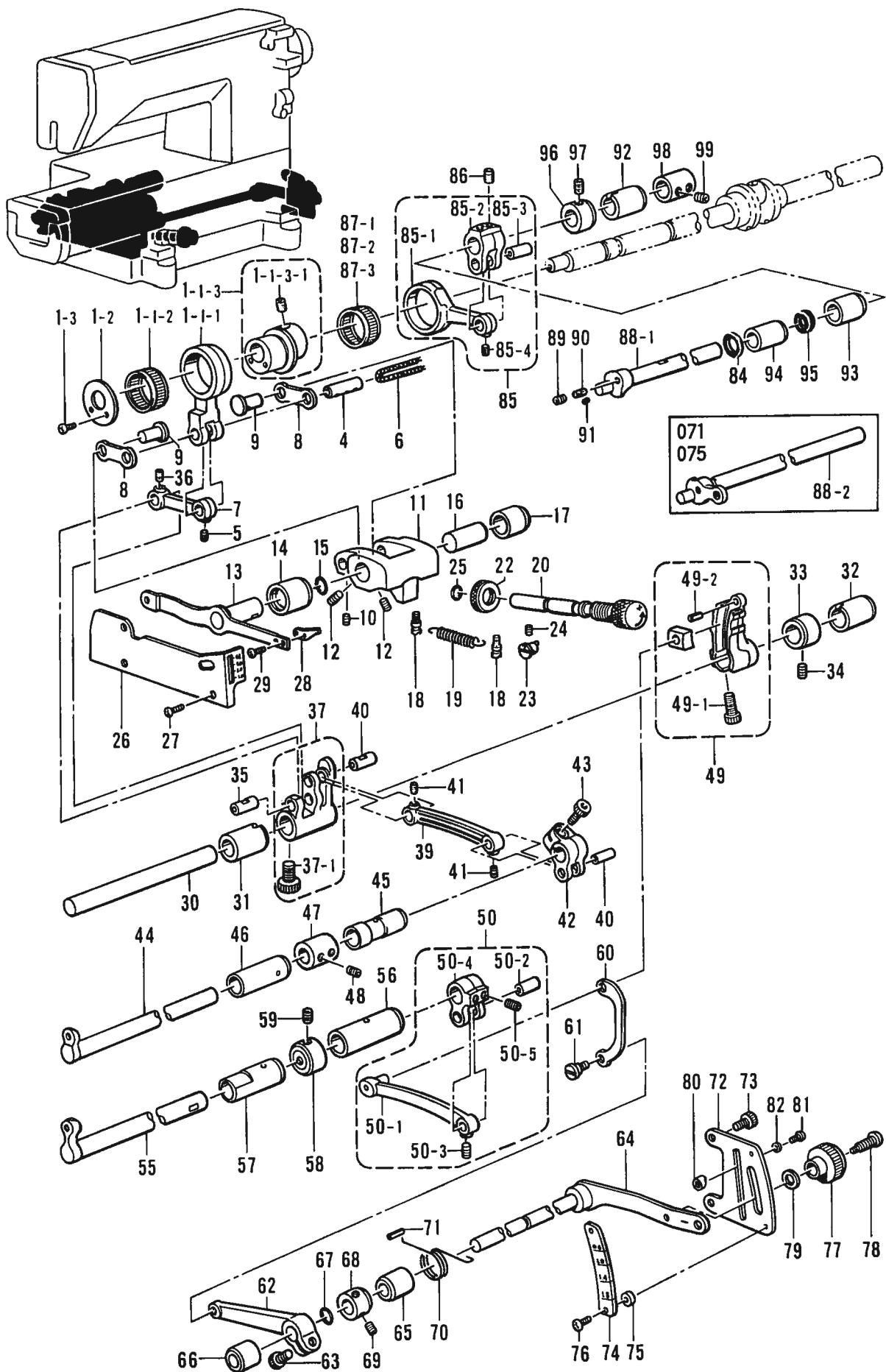
**E1. 送り関係 /Feed mechanism/Transportvorrichtung/
