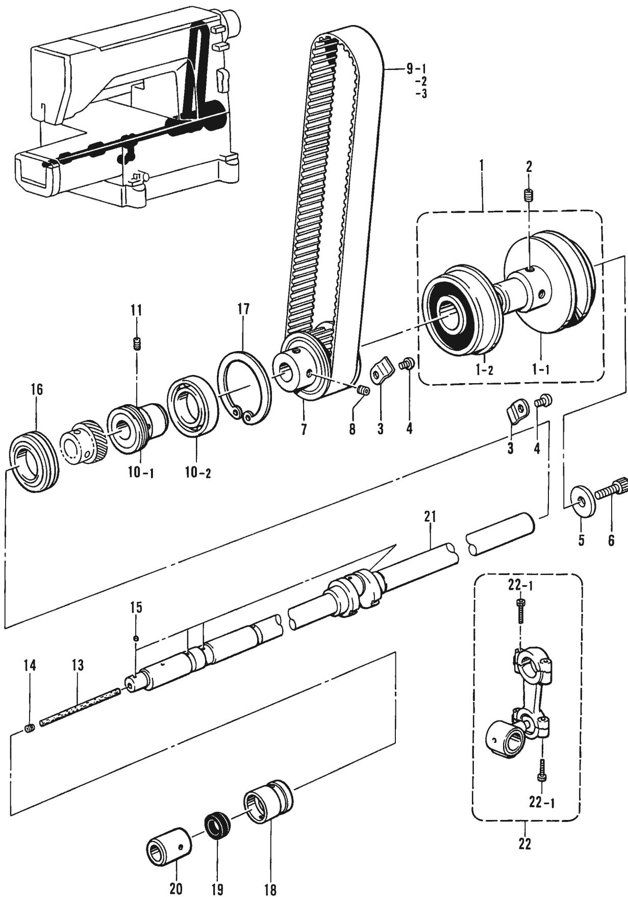
F. 下軸関係/Lower shaft mechanism/Untere Welle/
