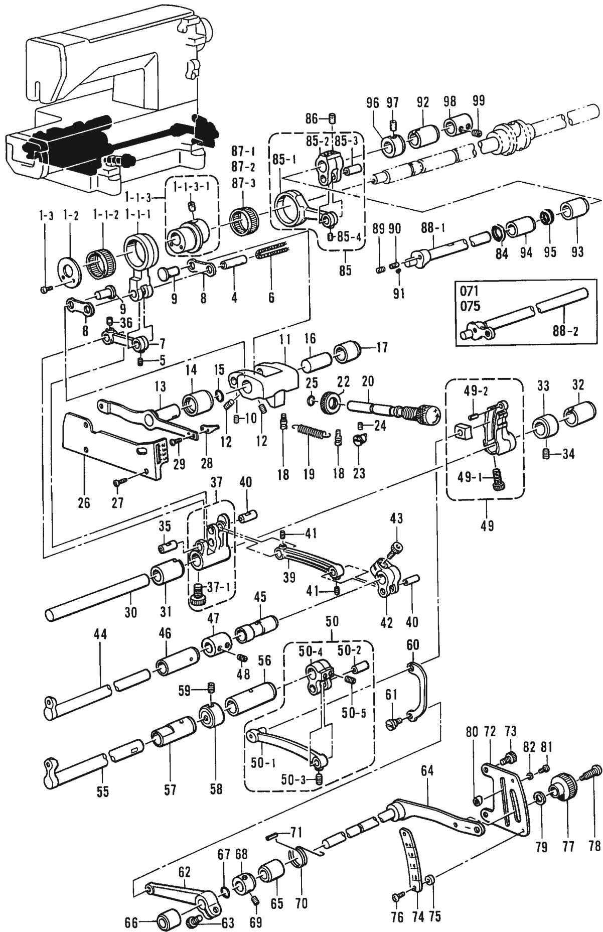
E1. 送り関係 /Feed mechanism/Transportvorrichtung/
