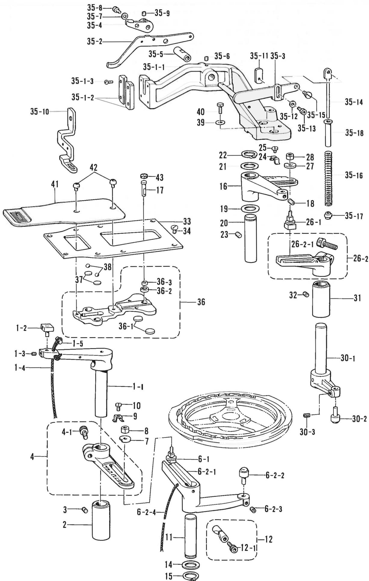
D. 送り関係 / Feed mechanism / Transportvorrichtung /
