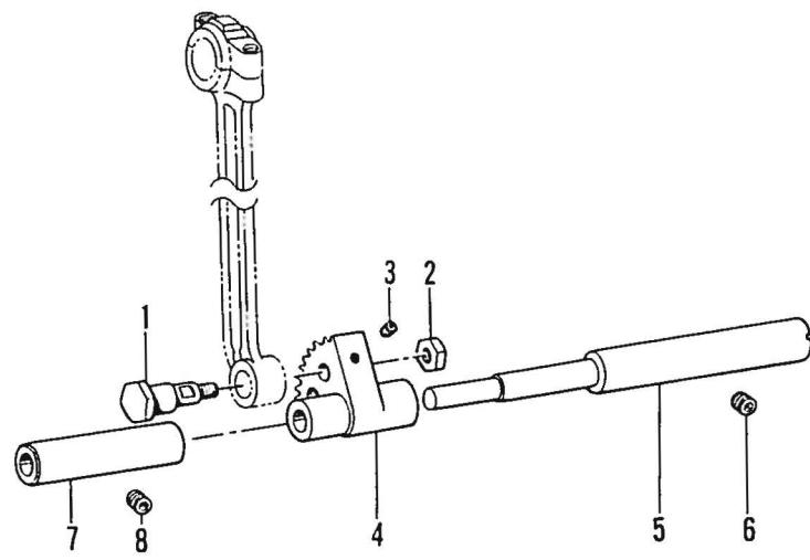
H. 下軸関係 / Lower shaft mechanism / Untere Welle /
