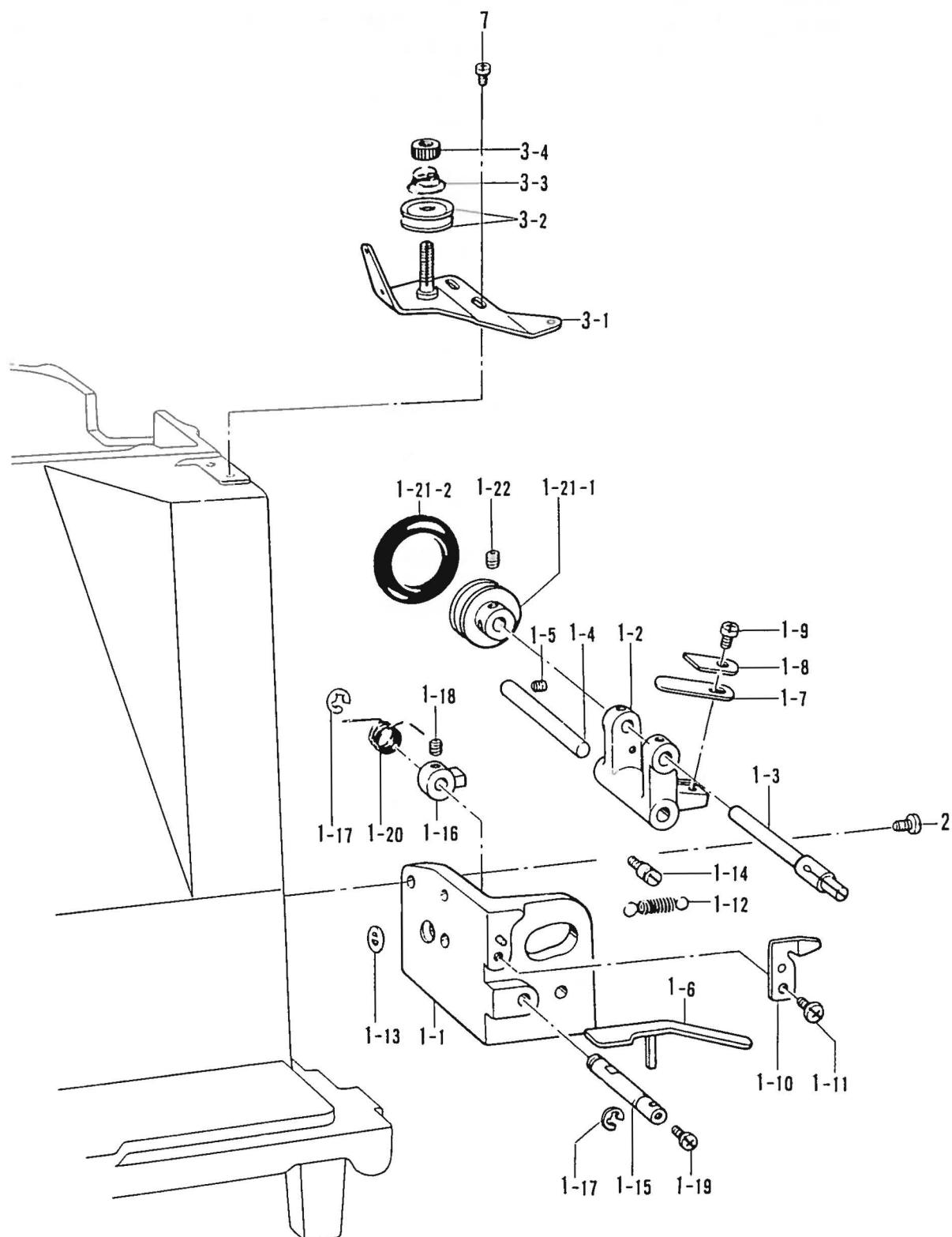
L. 糸巻キ関係 / Bobbin winder mechanism / Spuler /
