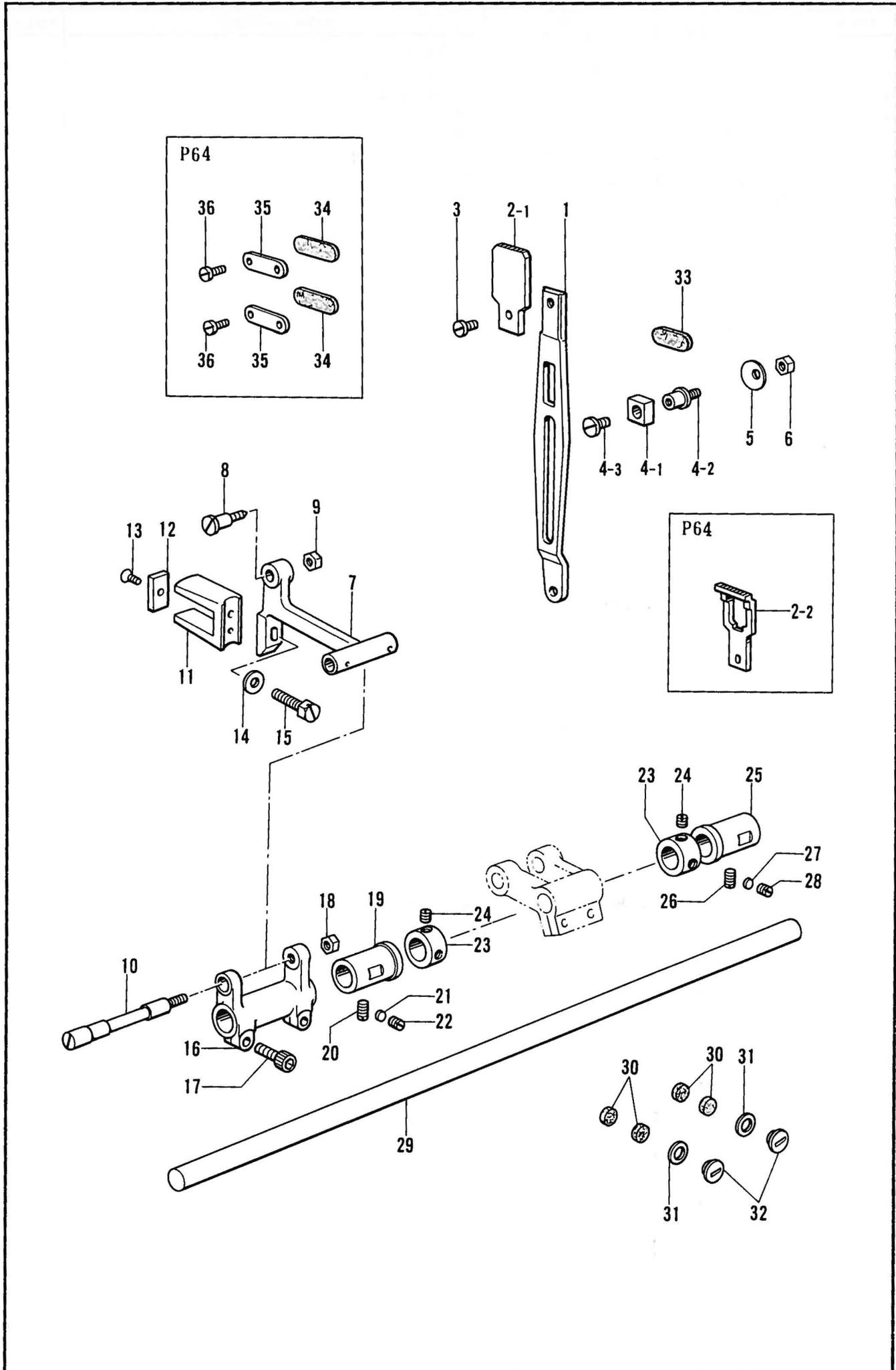
G. 送り軸関係/Feed shaft mechanism/Transport welle/
