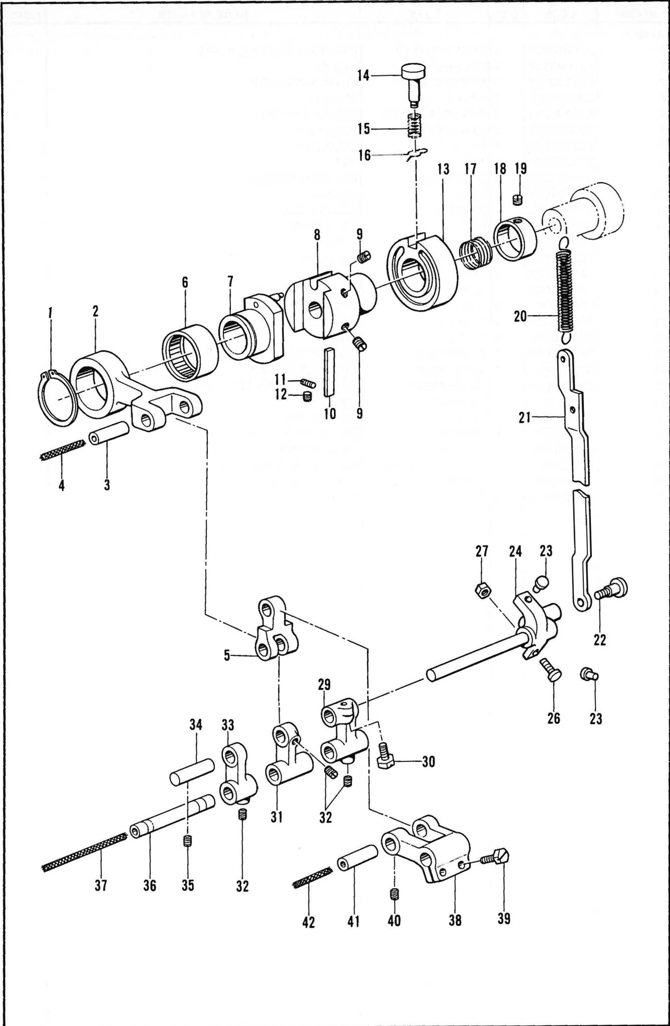
F. 送り関係/Feed mechanism/Transportvorrichtung/
