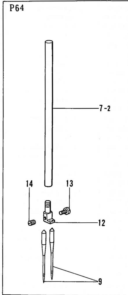
C. 針棒関係/Needle bar mechanism/Nadelstangenvorrichtung/
