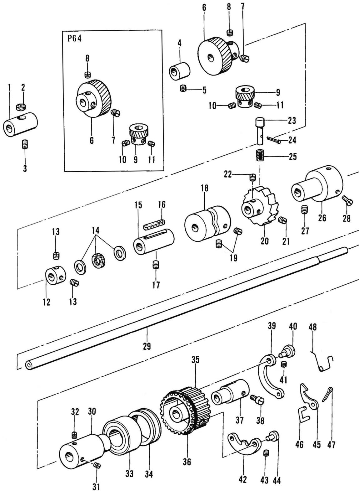
H. 下軸関係/Lower shaft mechanism/Untere Welle/
