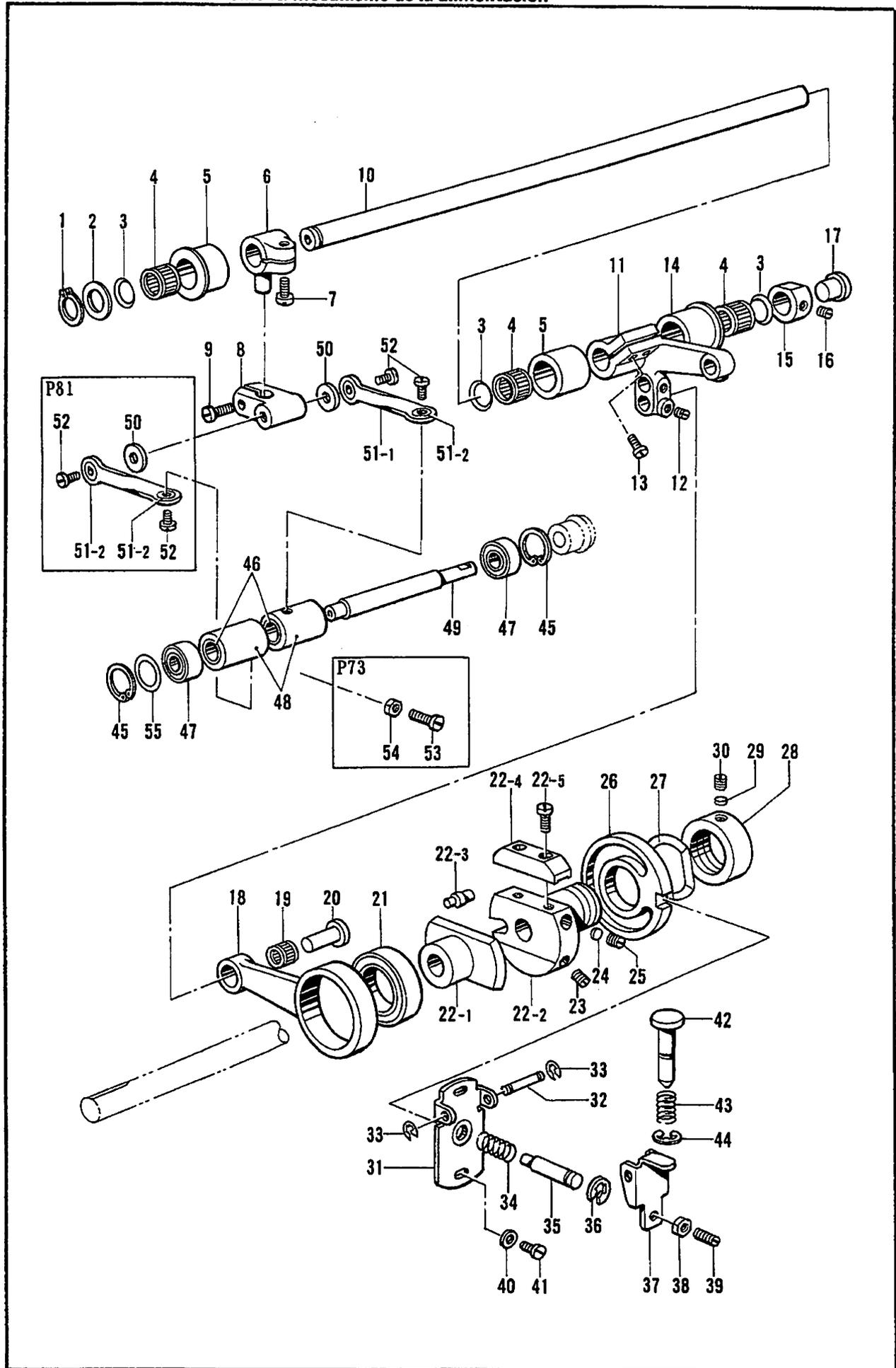
D. 送り関係/Feed mechanism/Transportvorrichtung/
