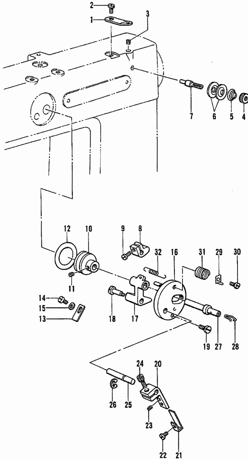
L. 糸巻キ関係/Bobbin winder mechanism/Spuler/
