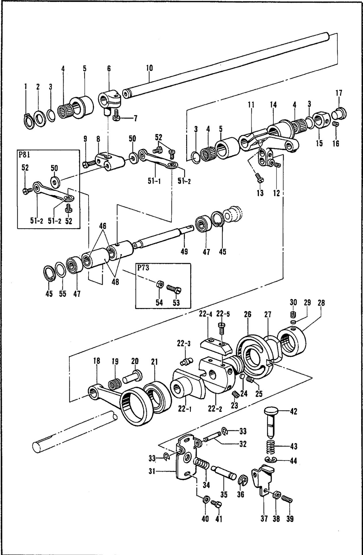
D. 送り関係/Feed mechanism/Transportvorrichtung/
