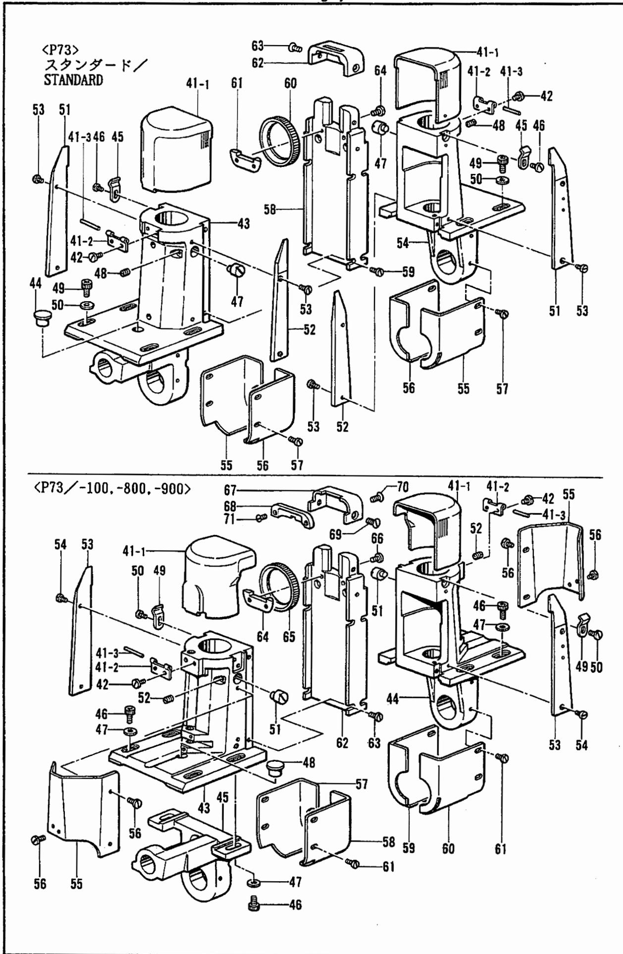
J5. カマ関係/Rotary hook mechanism/Greifervorrichtung/
