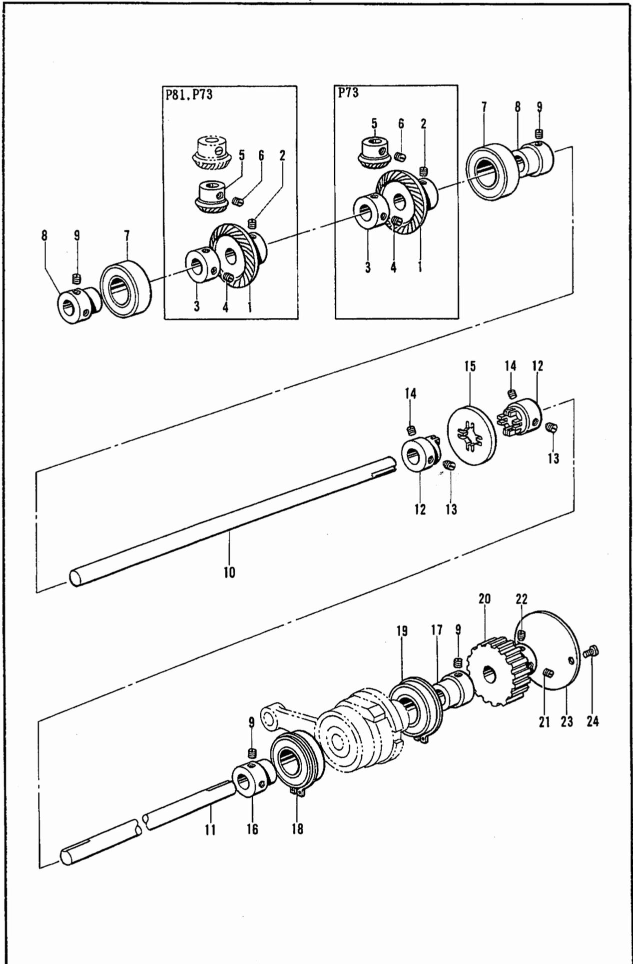
H. 下軸関係/Lower shaft mechanism/Untere Welle/
