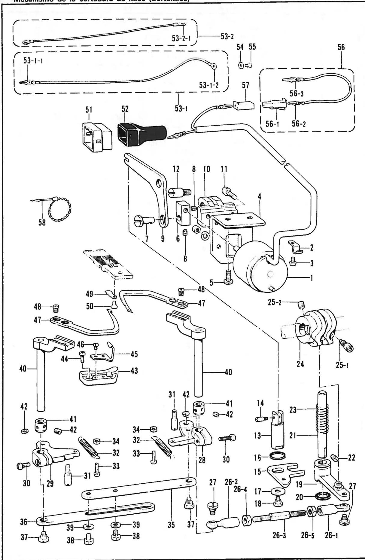
N. 糸切り関係 (糸切り) / Thread trimmer mechanism (Thread Trimmer) /
