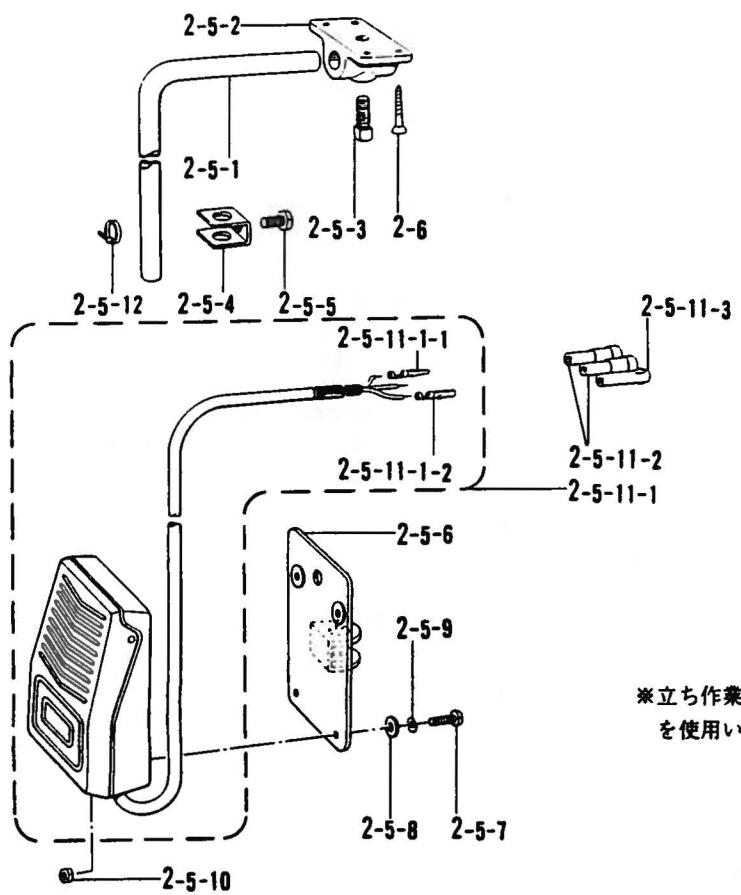
V2. 電磁押工上ヶ関係 (オプション)/Presser foot lifting solenoid set (Option Parts)/
