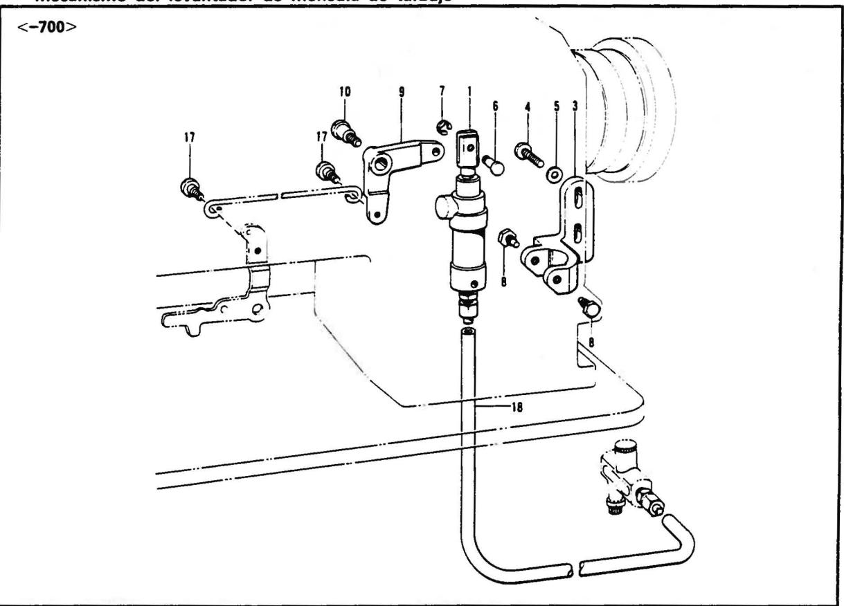
F. 送り軸関係/Feed shaft mechanism/Transport welle/
