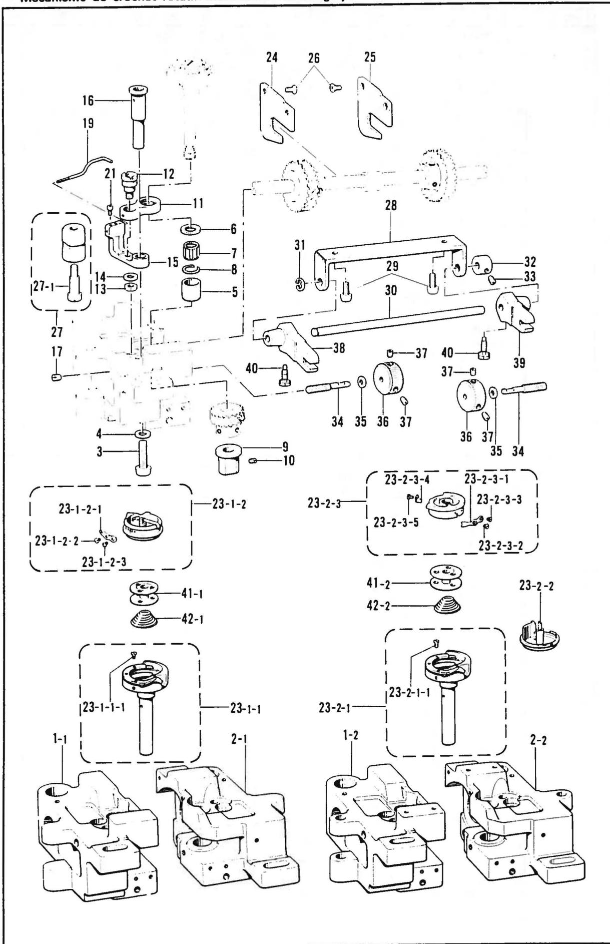
K. カマ関係/Rotary hook mechanism/Greifervorrichtung/
