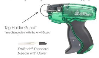
No. 11500 Standard Mark  $V^{TM}$  hand tool is most commonly used for tagging general-purpose and heavy-duty fabrics:
