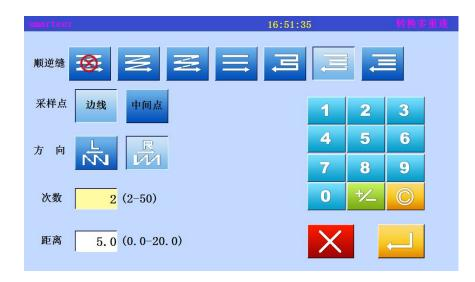
\* Select and input multiple layers of sewing, direction, distance, and number of times
