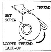
G. TO DECREASE THE AMOUNT OF LOOPER THREAD IN THE SEAM MOVE THREAD GUIDE EYELET TO ALIGNING MARK TO INCREASE, MOVE IT BACKWARD.
