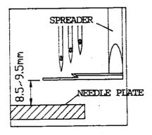
F. WHEN SPREADER MOVE TO THE LEFT AND PASSES BEHIND THE LEFT NEEDLE, THE CLEARANCE IS 0.5 - 0.8 mm. AND WHEN SPREADER REACHES THE EXTREME LEFT, THE DISTANCE BETWEEN TIP OF HOOKING PART AND THE CENTER OF LEFT NEEDLE IS 4.5 - 5.5 mm.
