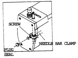
E. AFTER ADJUSTMENTS, TIGHTEN THE SCREW OF NEEDLE BAR CLAMP AND MAKE SURE THE NEEDLES ARE IN THE CENTER OF NEEDLE DROP HOLE OF NEEDLE PLATE.
