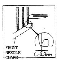
C. THESE ADJUSTMENTS CAN BE MADE BY LOOSENING SCREW (A) IN ORDER TO ADJUST THE ANGLE AND HIGH OF FRONT NEEDLE GUARD AND LOOSENING SCREW (B), THEN TURNING HAND WHEEL IN ORDER TO ADJUST THE PROPER POSITION FOR NEEDLE, LOOPER AND FRONT NEEDLE GUARD.
