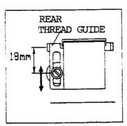
C. SOME TIMES, IT IS NOT SO EASY TO MAKE LOOP FOR SOME KINDS OF THREAD AND ALSO MAKE IT DIFFICULT FOR LOOPER TO CATCH THE NEEDLE THREAD, CAUSING SKIP STITCH. IN SUCH CASE, CAN USE AUXILIARY THREAD TENSION CONTROL GUIDE TO STABLIZE THE THREADS.
