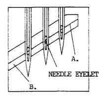
J/K. SETTING THE ANGLE AND TIMING OF REAR NEEDLE GUARD
