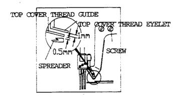
I. WHEN NEEDLE BAR AT THE LOWEST POSITION, THE CLEARANCE BETWEEN
