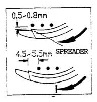
G. THE ADJUSTMENTS ARE MADE BY LOOSENING SCREW (A) FOR THE HEIGHT OF LOOPER AND LOOSENING SCREW (B) FOR MOVING POSITION OF LOOPER.
