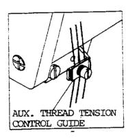
D. IN CASE THE FORMATION OF NEEDLE THREAD LOOP IS UNSTABLE WHEN USING STRECTCHABLE THREAD, YOU CAN SOLVE THIS BY ADJUSTING THE HEIGHT OF FRONT NEEDLE THREAD GUIDE, ESPECIALLY WHEN LOOPER MOVE FROM RIGHT TO THE LEFT.
