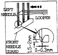
B. WHEN THE TIP OF LOOPER IS RETURNED TO THE KIGHT NEEDLE, PROVIDE A CLEARANCE OF 0 - 0.3 mm BETWEEN THE RIGHT NEEDLE AND FRONT NEEDLE GUARD.
