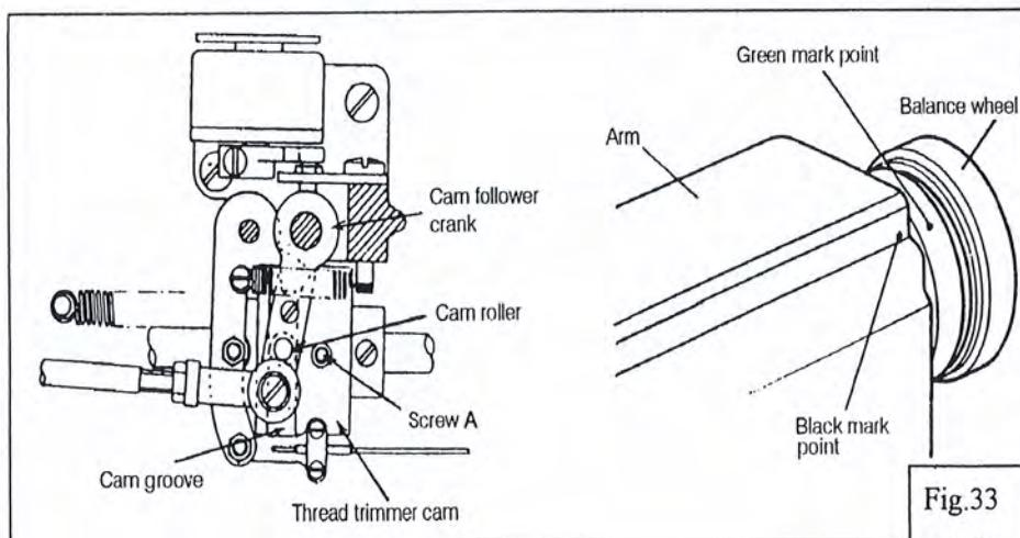
**Note:** To adjust, Loosen two thread trimmer cam clamp screws A.
