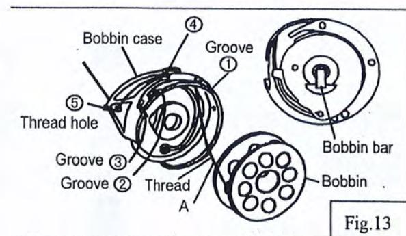
Leading the lower thread and install the bobbin
