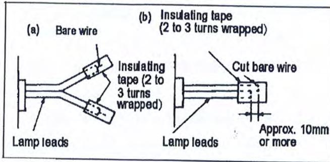
**CAUTION: The illuminating lamp must not be connected with any heater, such as a foot warmer and others, in parallel. Otherwise, the load capacity will be exceeded. It may cause transformer winding burned out.**
