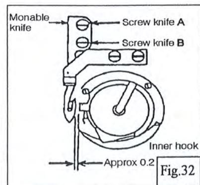
**B Gap between movable knife and bobbin case holder stopper (Fig.32)**
