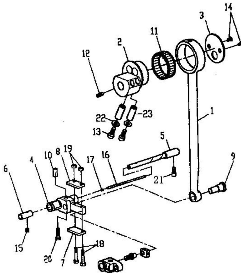
**F、下轴机构 HOOK DRIVING SHAFT COMPONENTS (2/2)**
