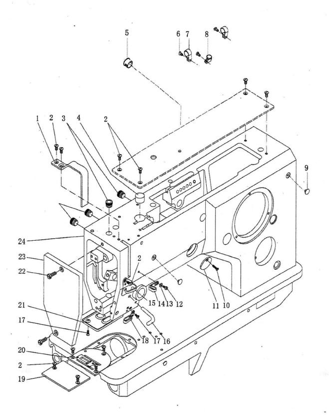
B. Brbbin winder and thread tension parts
