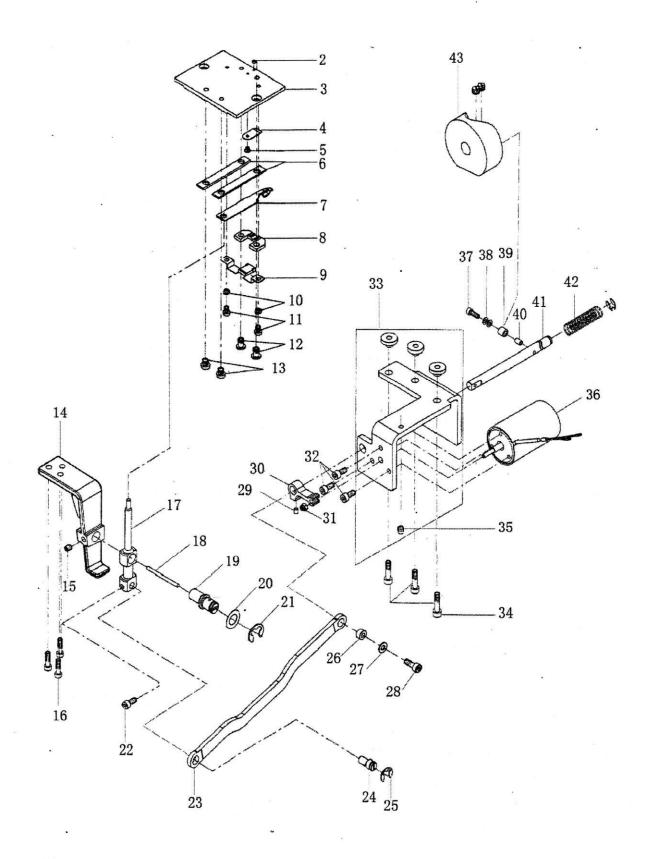
L. Tension release, electrocircuit board, oil circuit parts
