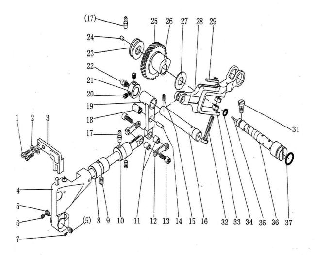
E. Needle bar vibrating parts
