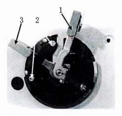
27 Lateral setting of straight stitches on throat plate needle hole edges, arresting of zigzag stitch setting mechanism
