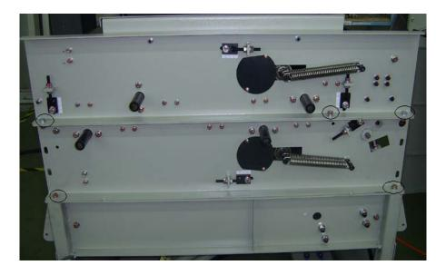
13. Remove 5 bolts fixing the upper and the lower frames.
