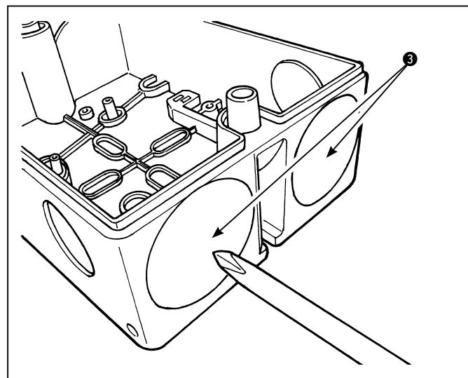
2) Make two holes, with a sharp instrument, in the center of grommet ③ located the lower part of the switch case.
