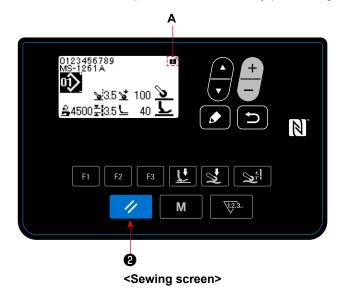
The status of the simple lock can be changed over between enable/disable by keeping // 2 held pressed for one second on the sewing screen.
