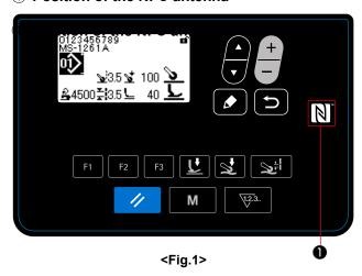
In the case of carrying out the NFC communication between the sewing machine and a tablet or smartphone, bring the antenna of the tablet or smartphone near to NFC mark ① as shown in Fig. 2.
