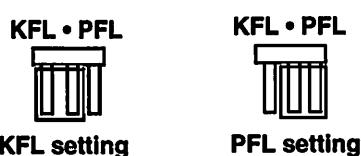
When the pedal sensor is changed (KFL → PFL or PFL → KFL), replace jumper ① to fit the pedal specifications changed.
