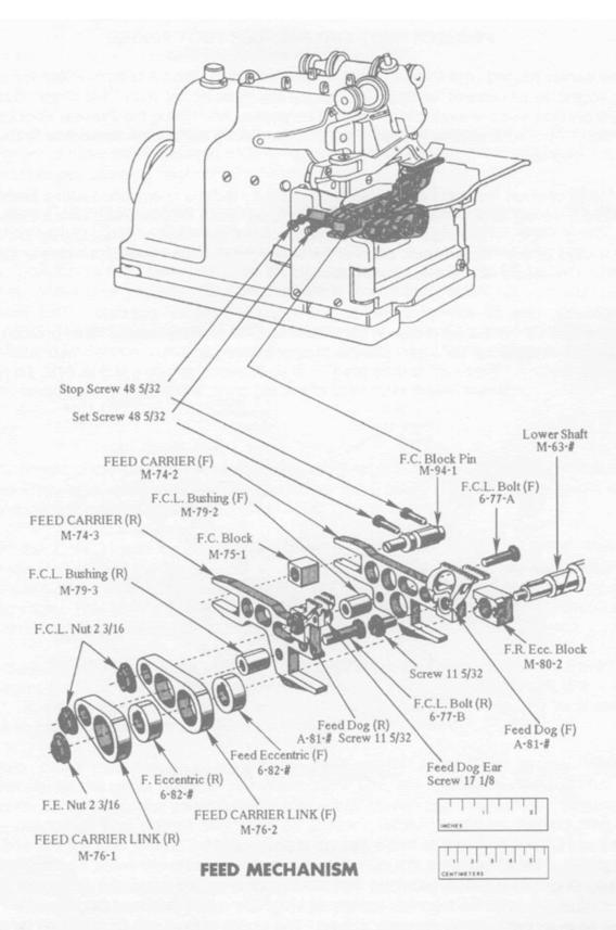
47. The Feed Dog and Needle Plate must match each other and it may be necessary to change Feed Dogs to prevent interference with the Needle Plate when very few stitches per inch are used.
