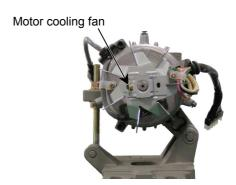
Fig. 3 Motor cooling fan mounting screw
