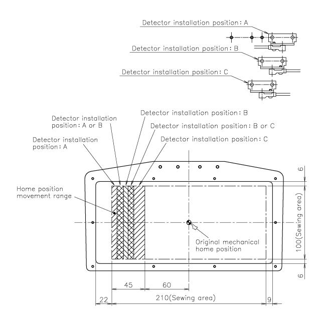
[Note] The shaded section below is the optimum range for moving the home position.
