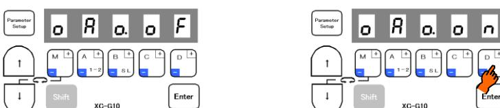
\* Output signal is turned ON while pressing the [D] key.
