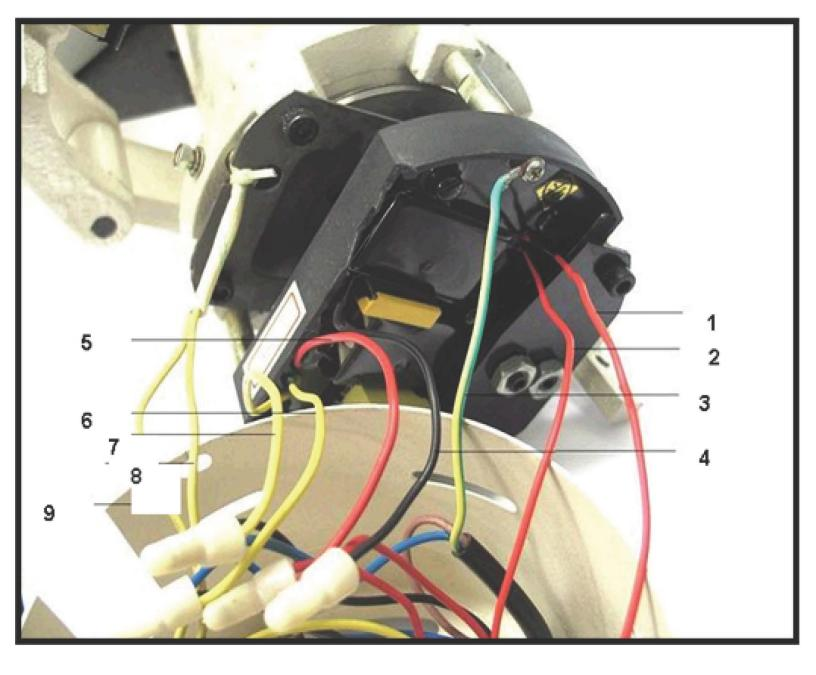
RED WIRES #1 & #2 Go to the Speed Control Potentiometer
