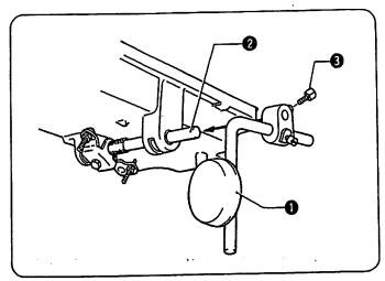
Place the knee lifter assembly • onto the knee lifter bar • on the oil pan, and then secure it by tightening the bolt 6.
