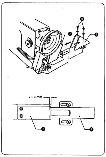
6. Place belt cover D ② so that it overlaps the belt cover ② by 2 − 3 mm, and then provisionally tighten the two screws ③.
