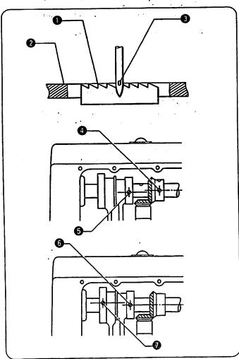
The standard timing is obtained when the feed dog • is lowered from its highest position until it is flush with the top of the needle plate 0, and the needle eye 0 is also aligned horizontally with these flush surfaces.
