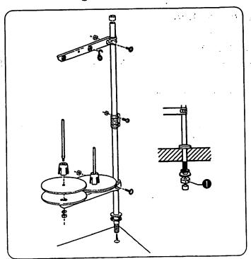
Assemble the cotton stand as shown in the illustration, and then install it to the work table.
