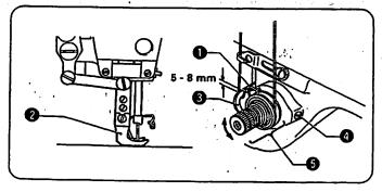
★ The standard position of the thread tension spring ① is 5 - 8 mm above the surface of the thread guide ② when the presser foot ② is lowered.
