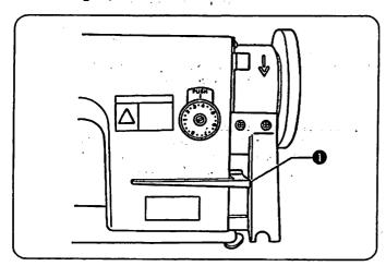
When the reverse stitching lever **①** is pushed, the cloth feed direction will be reversed, and when it is returned to its original position, the feed direction will change back to normal.
