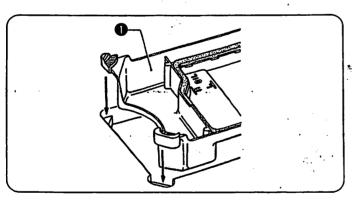
3. Place the oil pan 10 into the groove in the work table so that corners are aligned.
