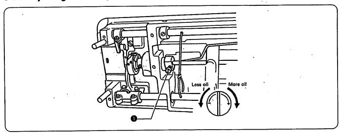
Tilt back the machine head, and then turn the oil adjusting screw • to adjust the lubricating amount.
