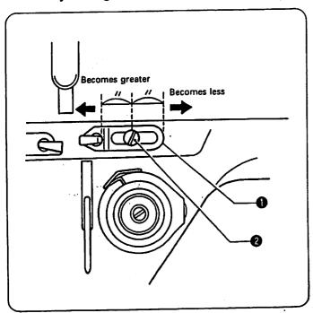
The standard position of arm thread guide R 10 is the position where the screw @ is in the center of the adjustable range for arm thread guide R 0.
