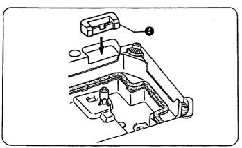
4. Insert the two rubber cushions • into the notches in the work table.
