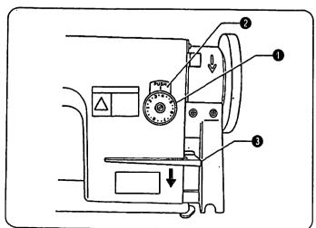
While pressing the stopper ②, turn the stitch length dial ① to the left and right to align the stitch length number with the reference line on the stopper ②.
