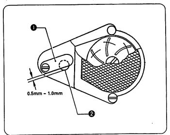
If you cannot see the oil being circulated by looking through the oil gauge window when the sewing machine is running at low speed, turn the oil adjusting plate • so that the oil hole • is covered.
