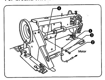
Connect the ground wire to the sewing machine head and motor.
