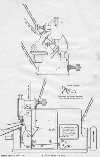
Threading for Three Thread Machines, Styles 60AB, 60ABD,
