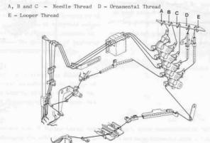
Note: The sketch hereabove shows the threading for 3 needle machines and the needle thread will be 2 for the 2 needle machines.
