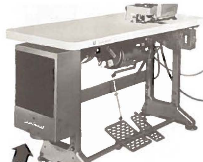
HEAT DISPELLER —Union Special's auxiliary unit (arrow) is an effective means for reducing oil temperature where heavy duty service requires it. Style 2899 E-1
