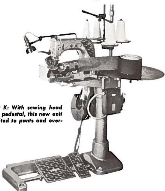
**STYLE 54200 K:** With sewing head overhanging pedestal, this new unit is ideally suited to pants and overall banding.
