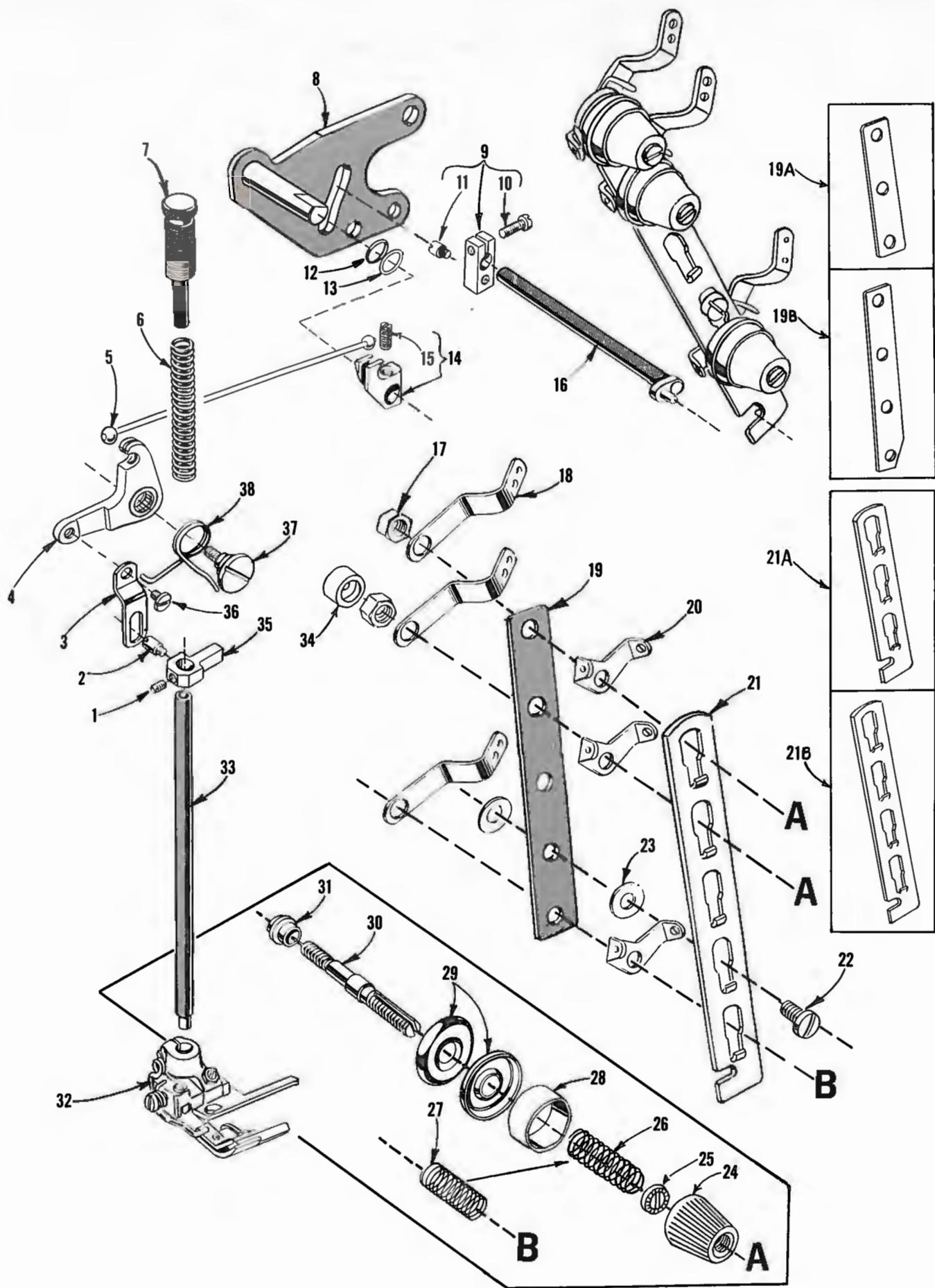
THREAD TENSION AND LIFTER LEVER PARTS
