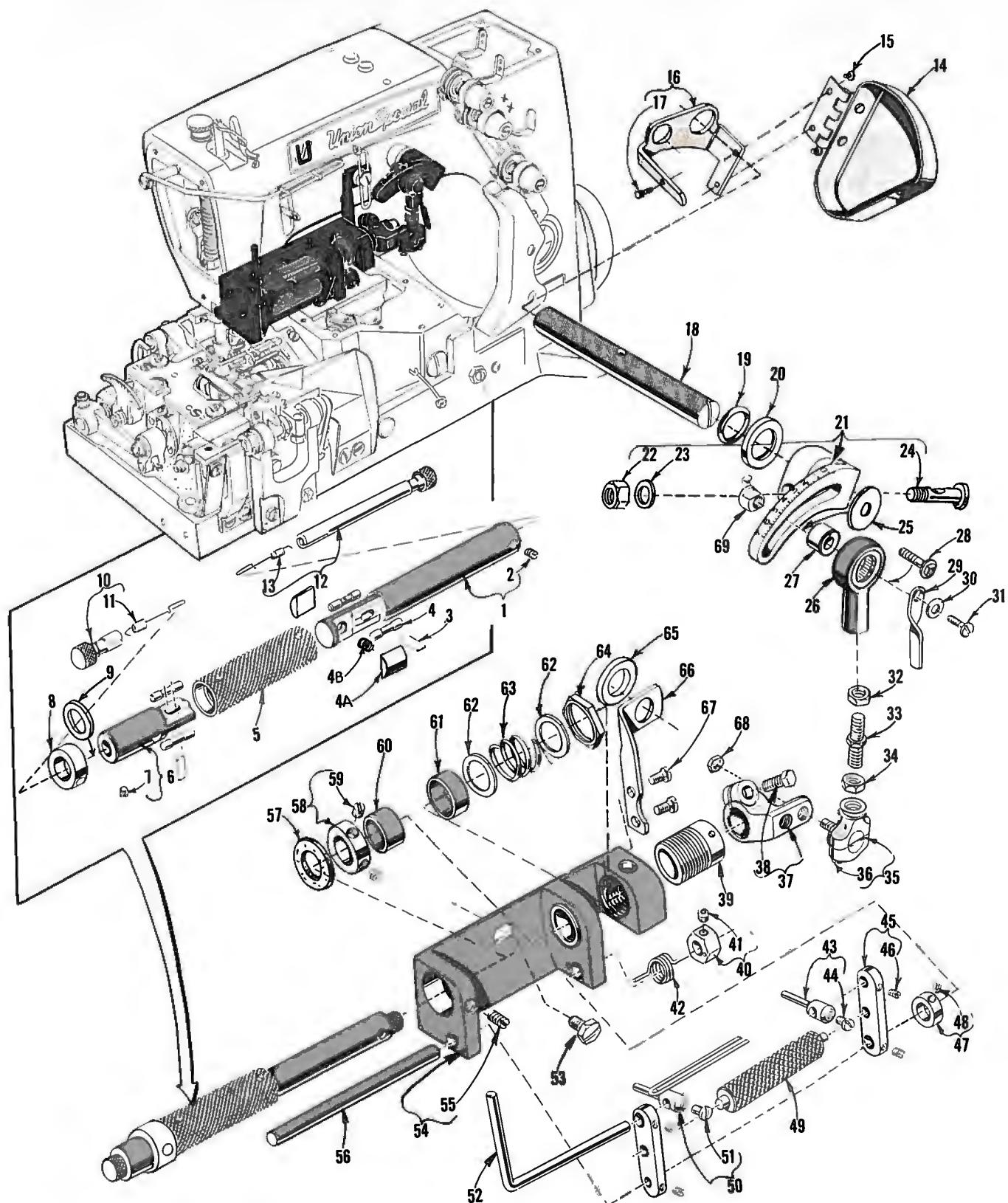
UPPER METERING DEVICE AND DRIVING PARTS
