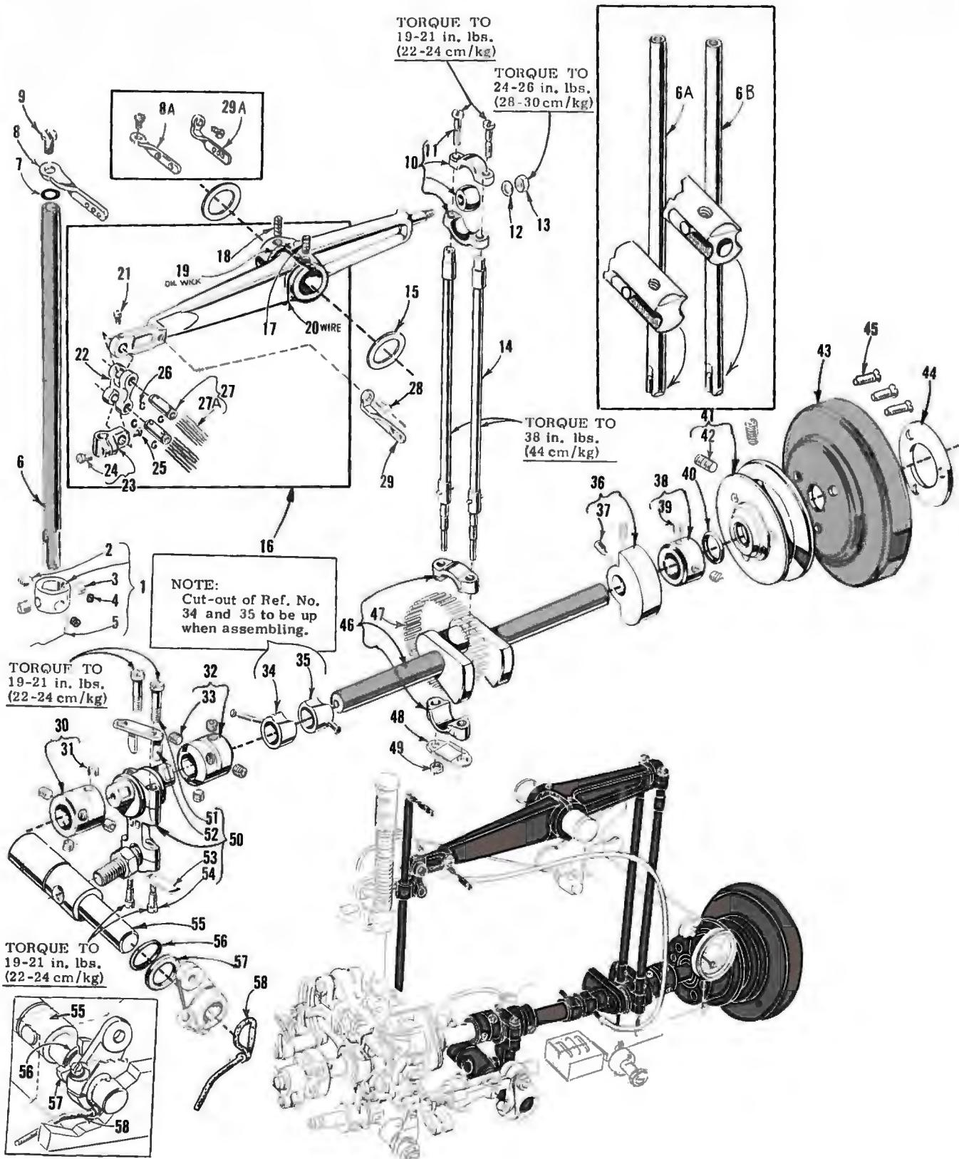
CRANKSHAFT, NEEDLE LEVER, NEEDLE BARS AND LOOPER DRIVING PARTS
