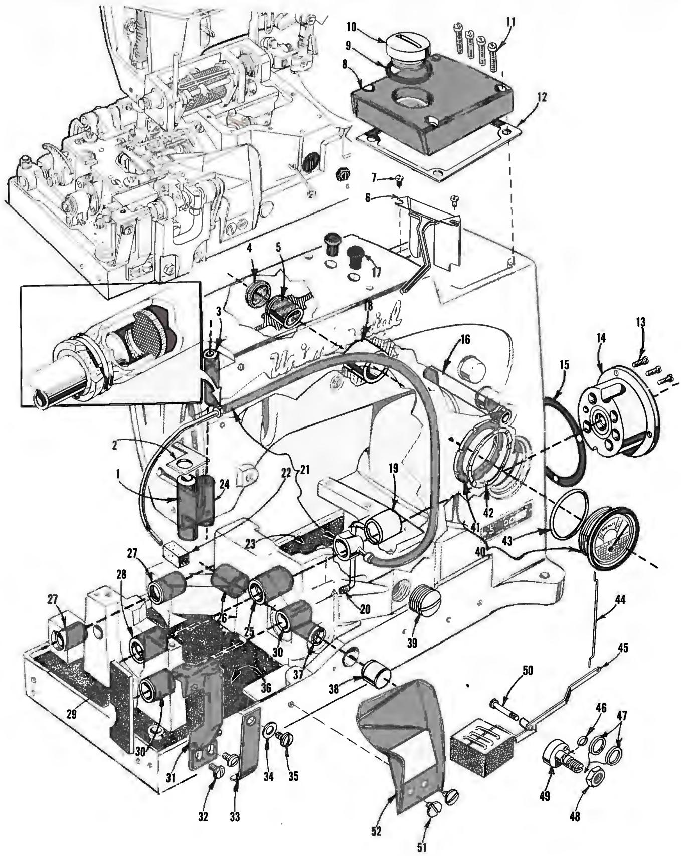
MAIN FRAME, BUSHINGS, OIL GAUGE AND MISCELLANEOUS OILING PARTS
