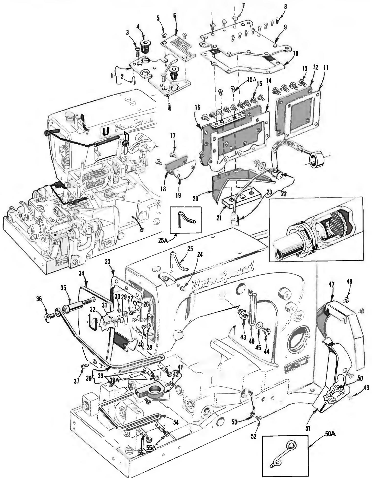
MAIN FRAME, MISCELLANEOUS COVERS AND OILING PARTS
