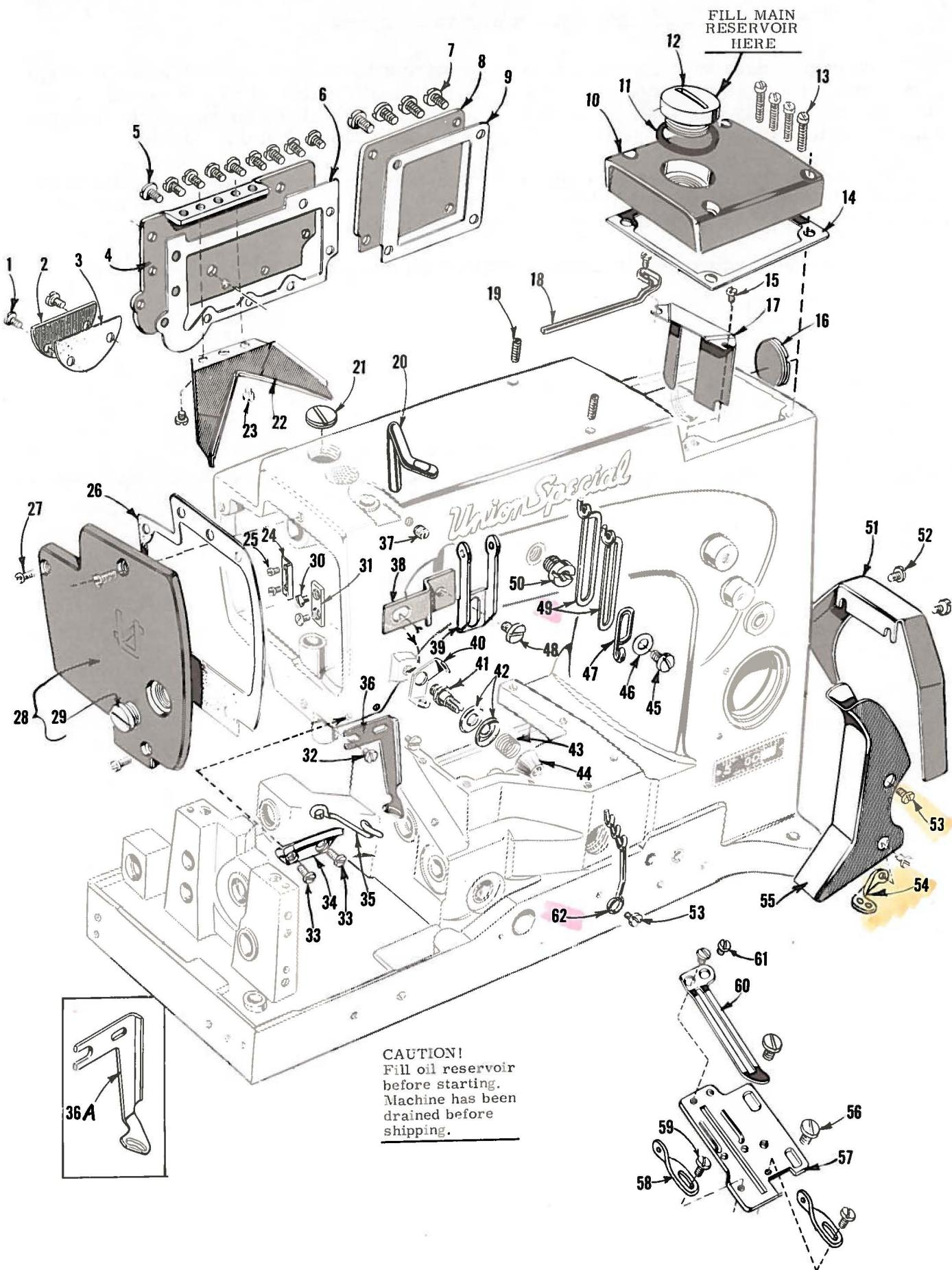
MAIN FRAME, CAST-OFF PLATE AND MISCELLANEOUS COVERS
