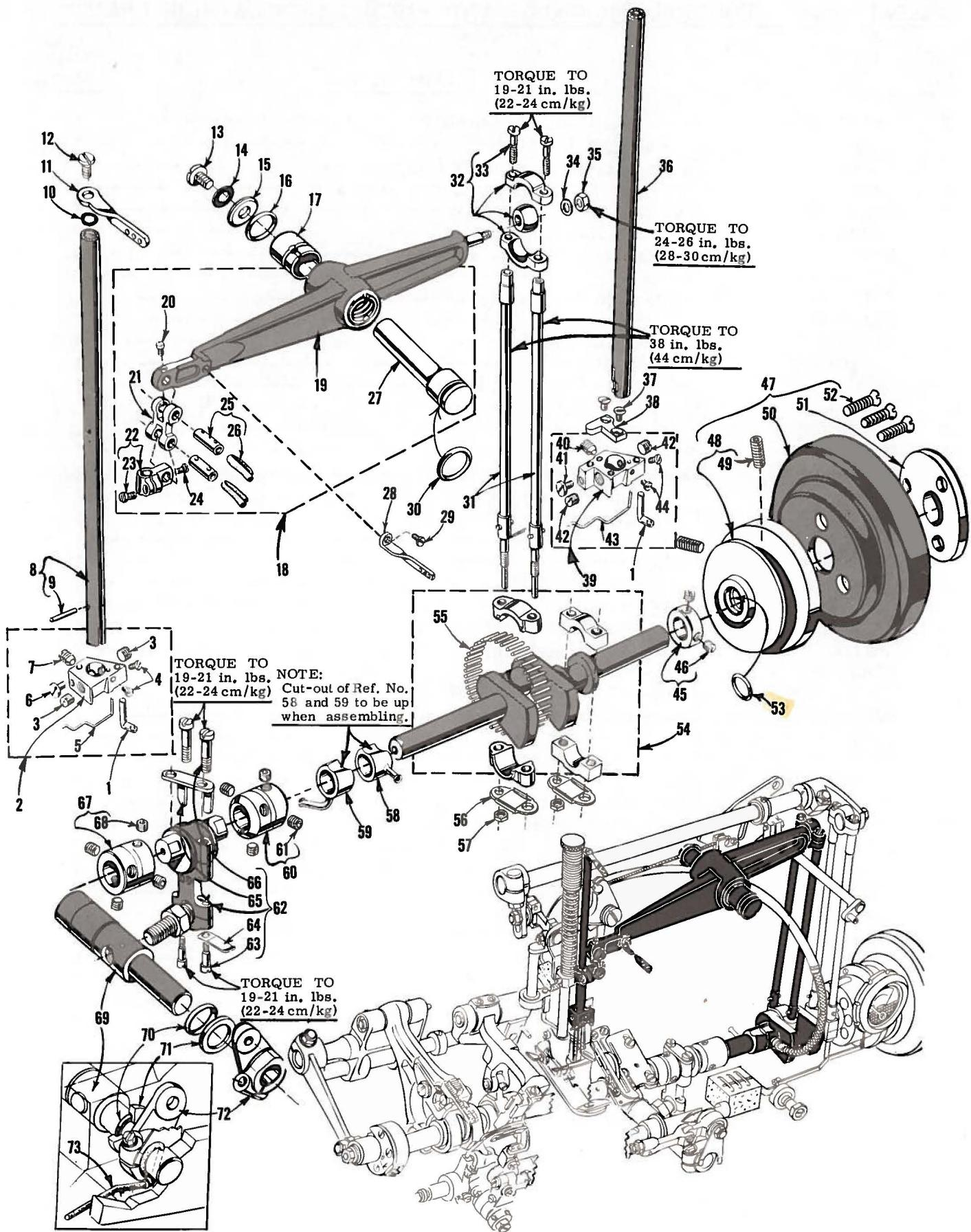
**CRANKSHAFT, NEEDLE LEVER, NEEDLE BAR AND LOOPER DRIVING PARTS**
