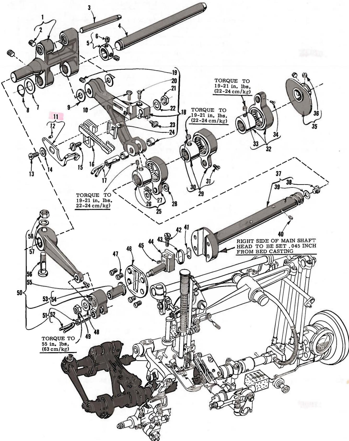
**NEEDLE GUARD, MAIN SHAFT, TAKE-UP AND FEED DRIVING PARTS**
