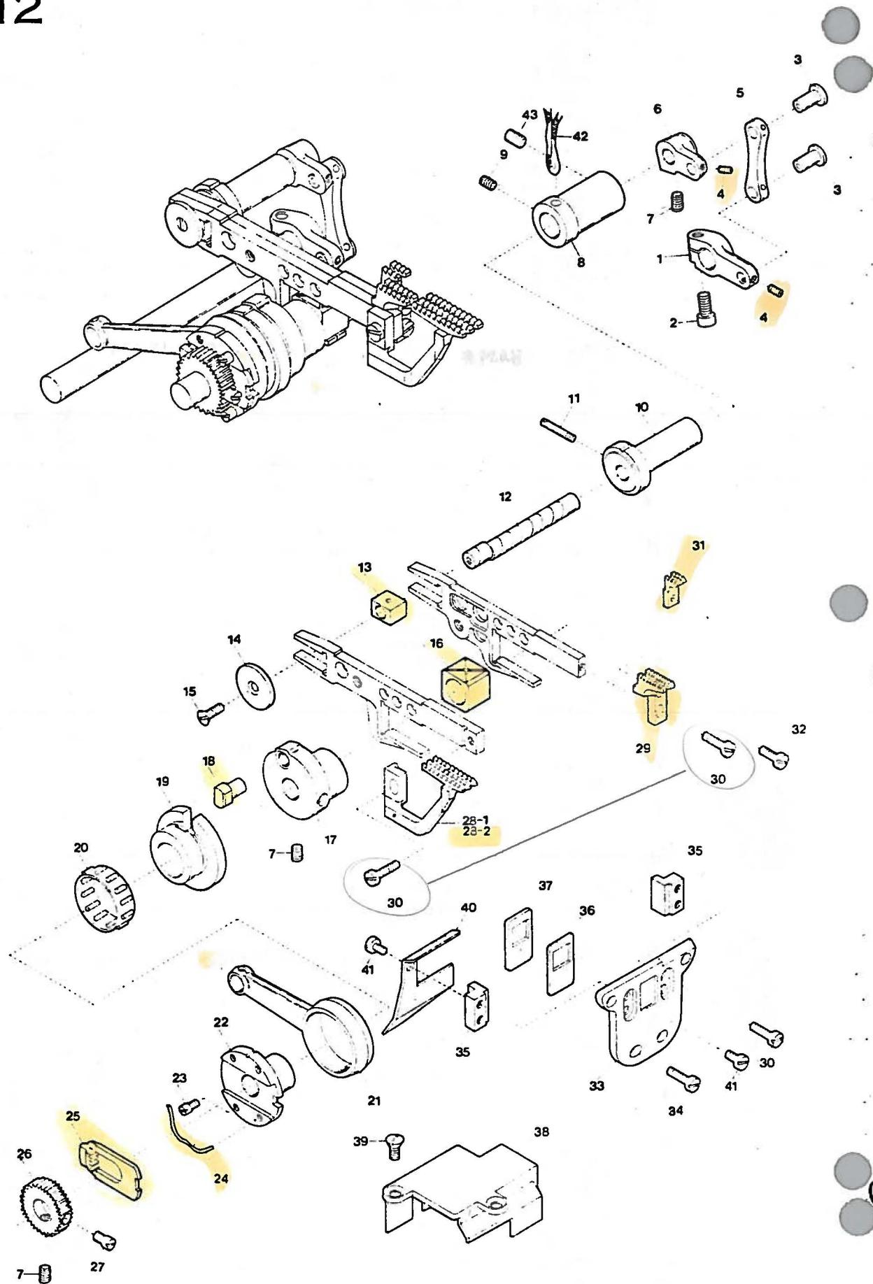
FEED DRIVING MECHANISM送り機構
