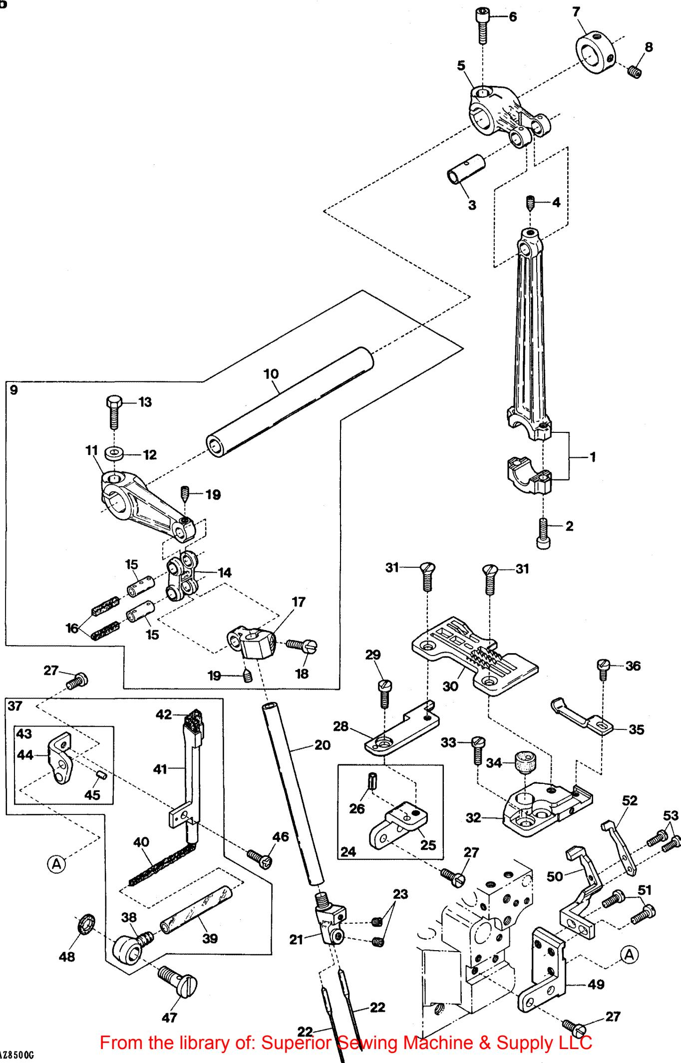
NEEDLE BAR DRIVING MECHANISM
