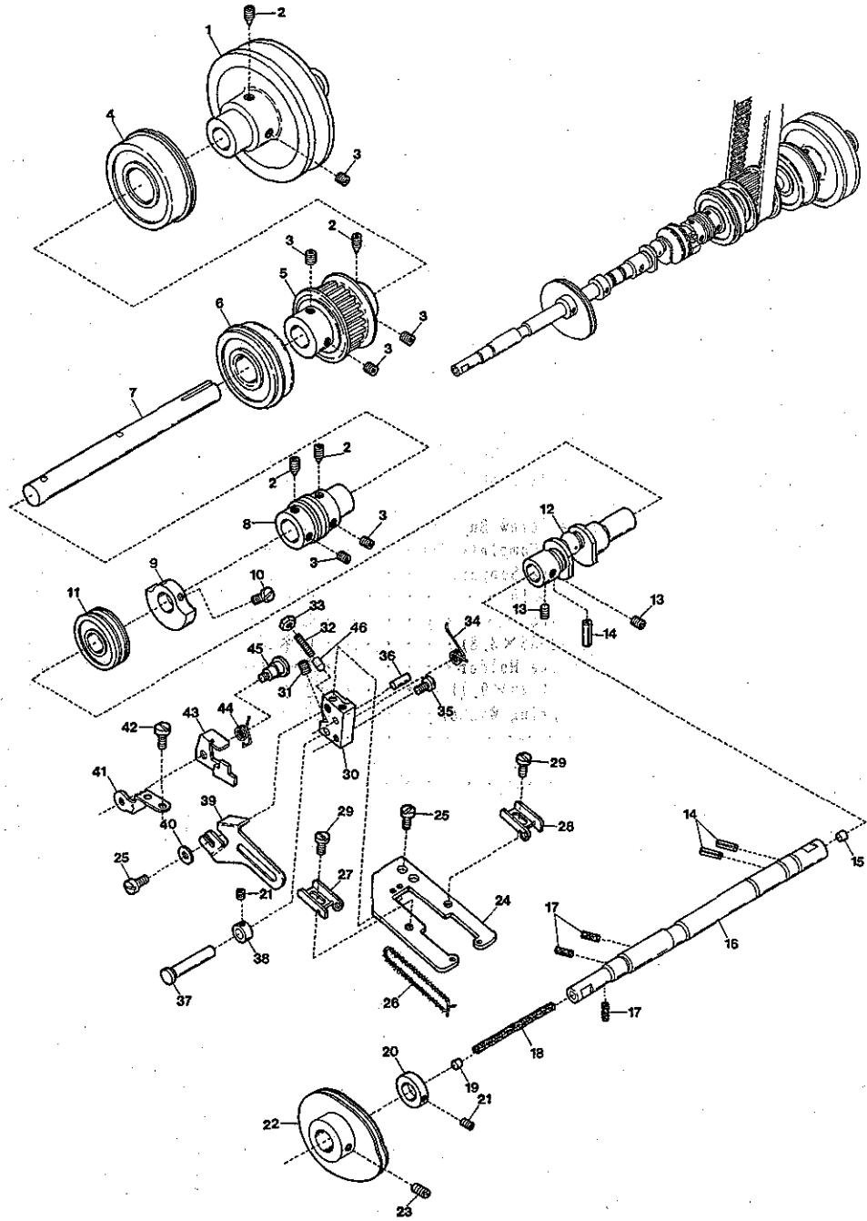
MAIN SHAFT DRIVING MECHANISM
