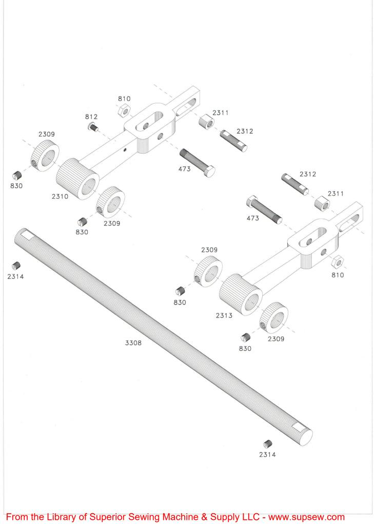
PARTS FOR ACE STRIP CUTTER MODEL C300WS PART NUMBER DESCRIPTION 473 810 Rod Pin Nut 812 Screw 830 2309 Screw Collar 2310 2311 2312 Rocker Lever Side Bushing Rocker Lever Pin Rocker Lever 2313 2314 Screw Rocker Lever Shaft 3308
