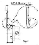
With the machine in this position, rotate the hook on its shaft until the hook point coincides exactly with the center line of the needle. Lightly lock the hook set screws on the hook shaft. At this position raise or lower the needle bar (in case B remove the clamp used) until there is a distance of 0.5-1.5 mm between the hook point and the upper edge of the needle eye (Fig. 3). Now clamp the needle bar in this position. The hook must now be set in its transverse position.
