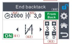
Long press key (3) in main interface or long press key (41) in fixed stitch interface to enter setting interface.
