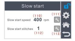
In order to ensure the thread picking and nipping stability of next sewing step after trimming, soft start function can be turn on.
