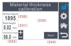
Press foot height detector installed or position changed, must calibrate again.
