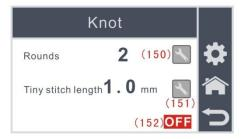
When used tie thread, can reduce the bird's nest.
