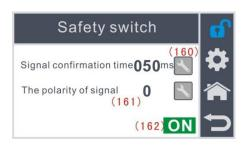
To prevent any wrong motion from machine head vibration, motion will be confirm after signal changed for a while, (160) adjusting confirmed time;
