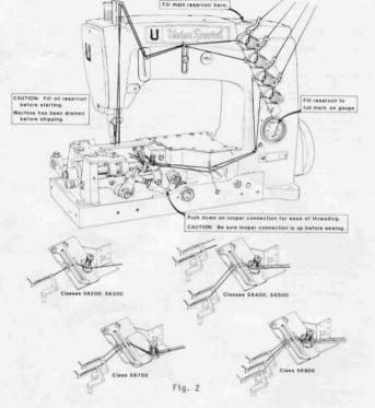
THREADING AND OILING DIAGRAM
